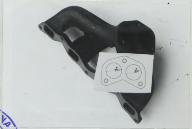
Q. exhaust manifold
