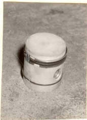
Photograph of piston showing crown to be affixed here.
