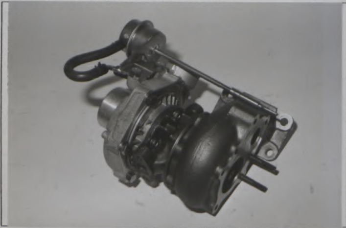
O) Valve and by-pass installation of turbocharger 過給圧調整装置
