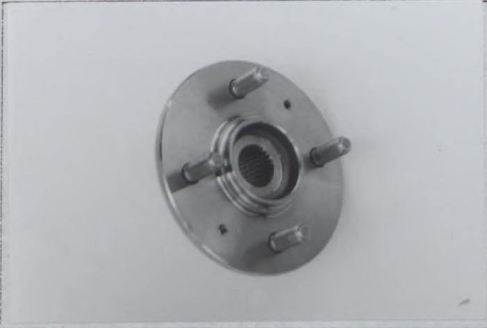
Photo V3 Reinforced front hub
