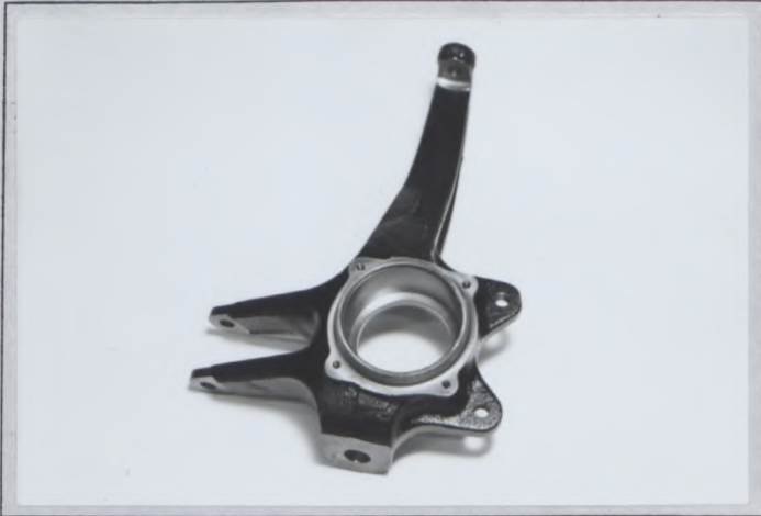
Photo T7 Heavy duty knuckle
