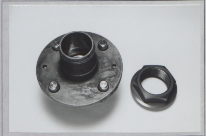
Photo T19 Rear hub for center lock
