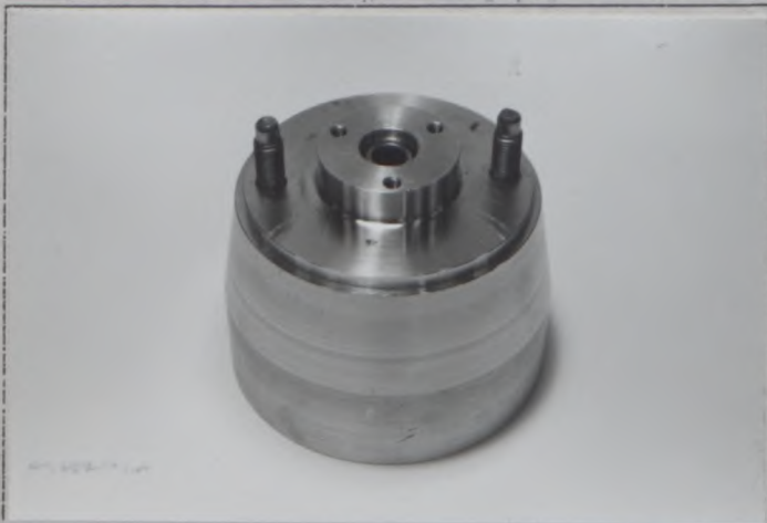
Photo T5. Reinforced rear damper mount
