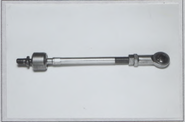
Photo T17 Reinforced steering tie-rod
