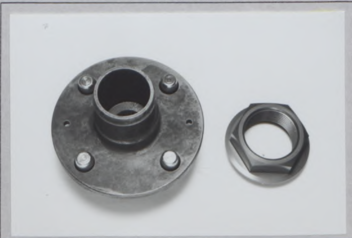
Photo T18 Front hub for center lock
