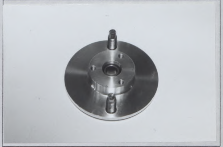
Photo T14 Reinforced rear damper mount
