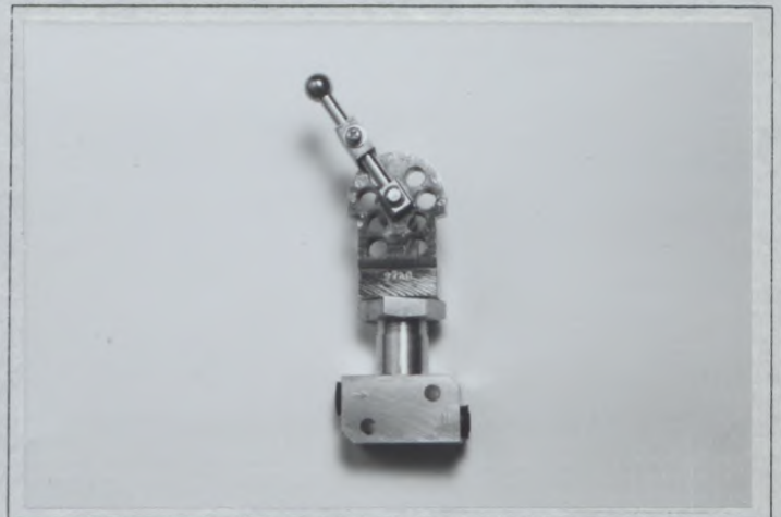
PHONT W2: BRAKING ADJUSTER
