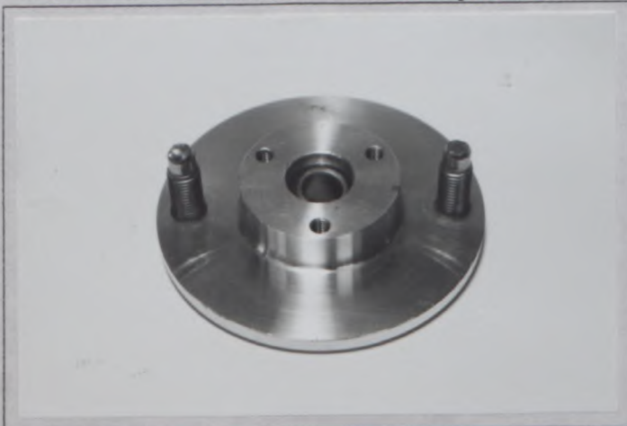
Photo T5 Reinforced front damper mount
