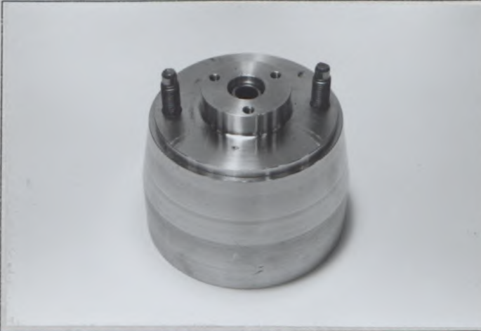
Photo T1. Reinforced front damper mount
