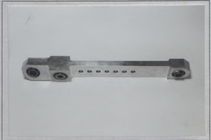
Photo T12 Reinforced rear lower arm
