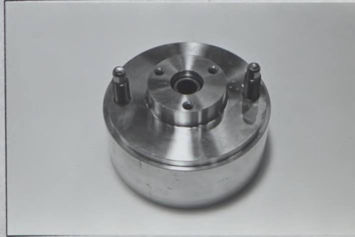
Photo T10: Reinforced rear damper mount
