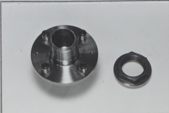
Photo T11: Front hub for center lock
