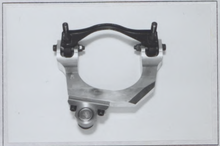
Photo T2 Reinforced front upper arm
