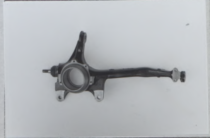
Photo V4 Heavy duty front knuckle
