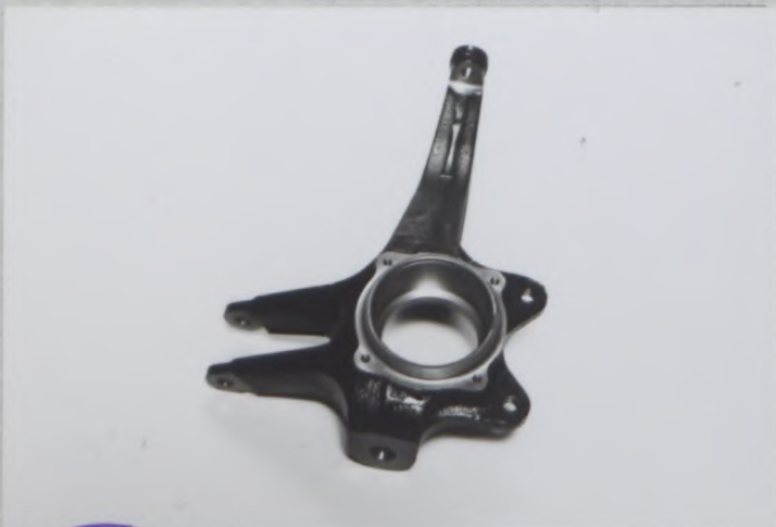
Photo T5. Heavy duty knucle
