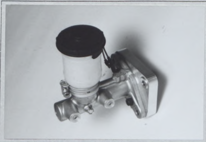
PHONT W1: BRAKE MASTER CYLINDER
