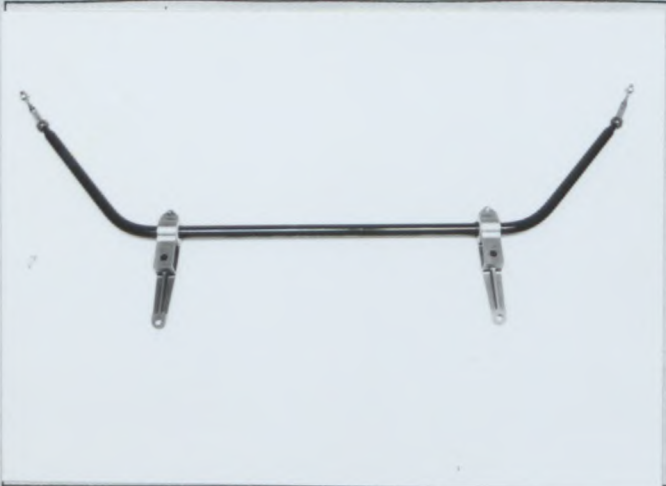
PHOTO 1 STABILIZER WITH LINKAGE, FRONT
