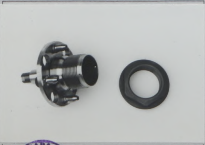
PHOTO U6 CENTRAL WHEEL BOLTING SYSTEM
