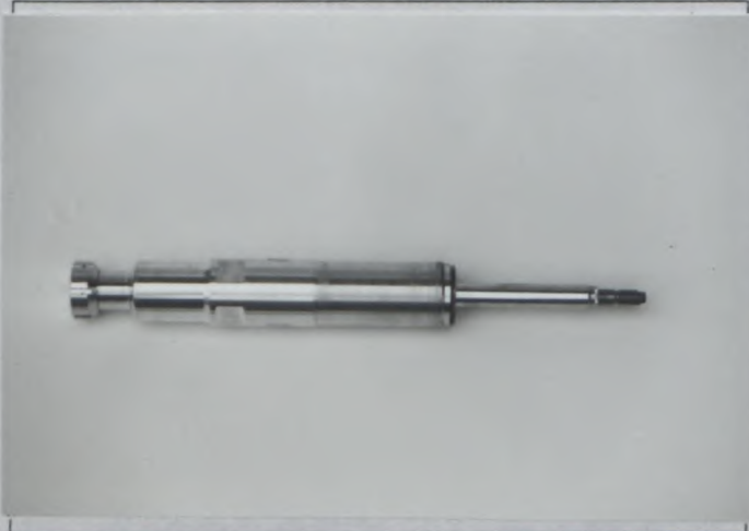
PHOTO U4 REINFORCED REAR STRUT
