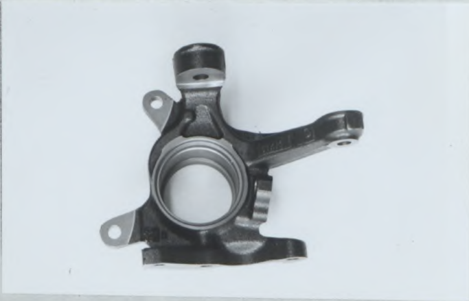
PHOTO T2 REINFORCED KNUCKLE (STD)
