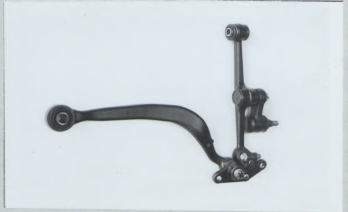
PHOTO T3 REINFORCED LOWER ARM (STD)
