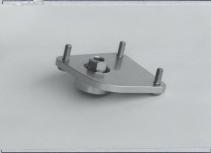
PHOTO U2 REINFORCED TOP MOUNT
