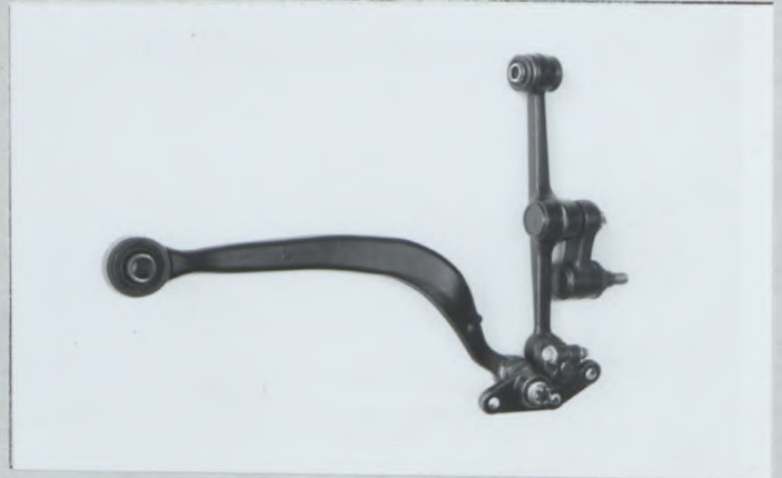
PHOTO T3 REINFORCED LOWER ARM (STD)
