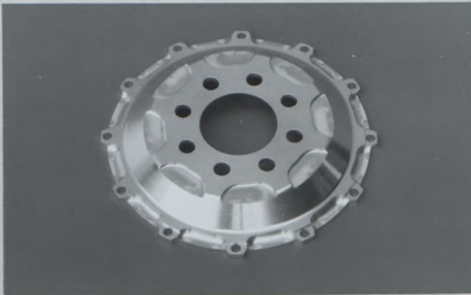
PHOTO V3 FRONT BRAKE BELL, TYPE D
