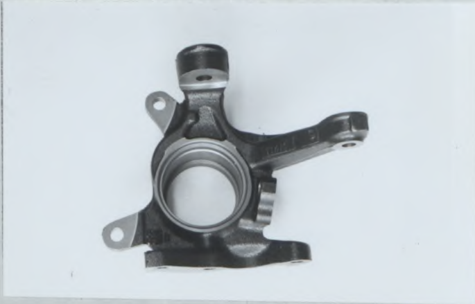
PHOTO T2 REINFORCED KNUCKLE (STD)
