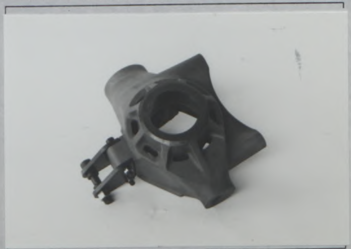
PHOTO T6 REINFORCED KNUCKLE TYPE A
