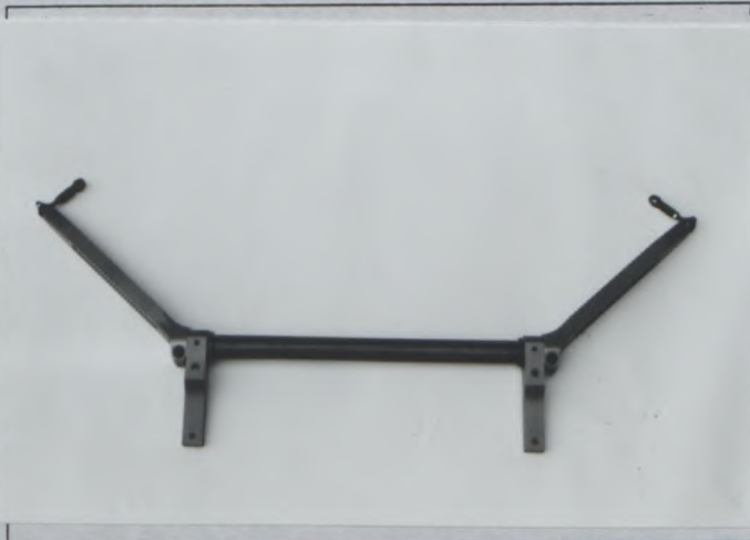
PHOTO T9 STABILIZER WITH LINKAGE
