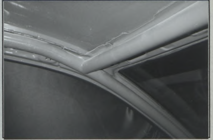
FRONT HOOP TO ROOF AND PILLAR
