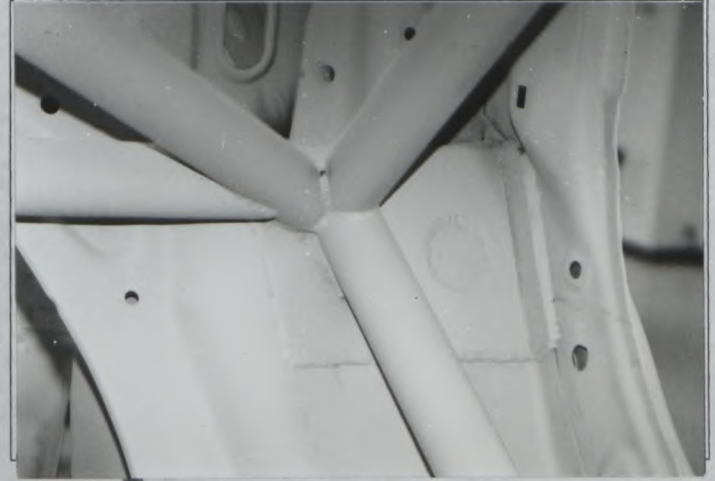
Photo No.4 Rear support to turret
