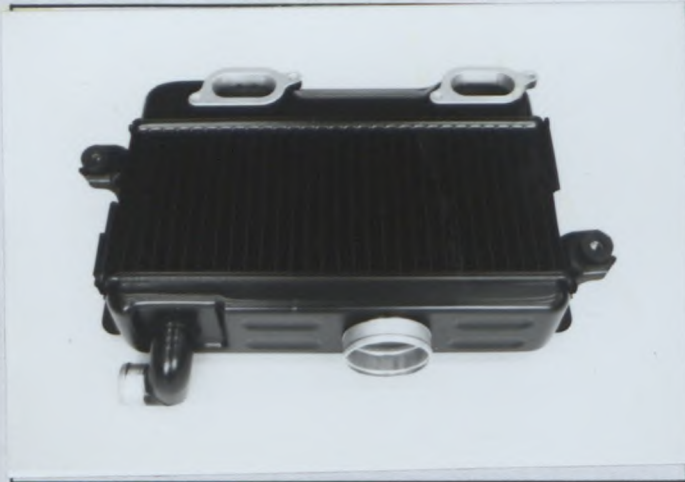
Photo R) Intercooler dismantled
