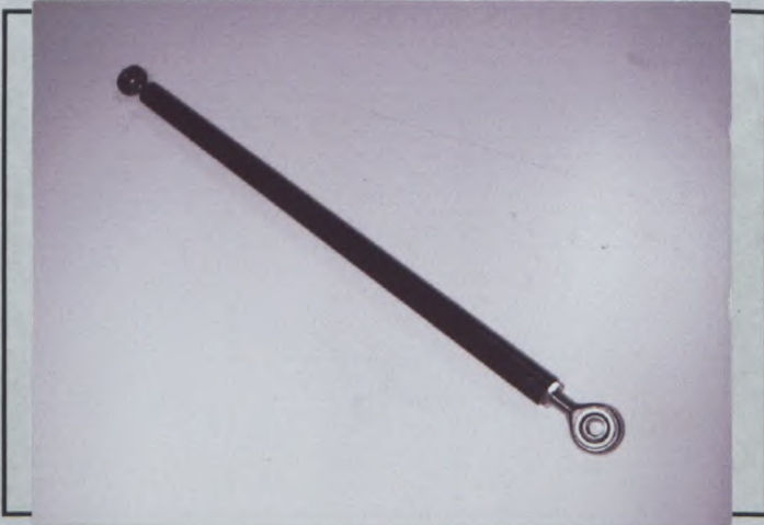
PHOTO N° 9: Steering column support
