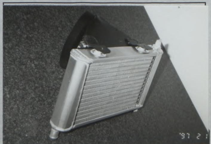
Photo 2) Alternative radiator and fixing for water cooled brake system
