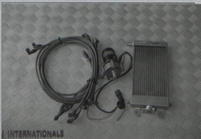
Photo 12) Water cooled brake system with pump , radiator and pipes
