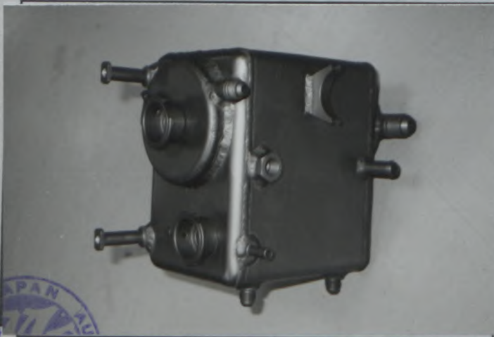
Photo 11) Water Cooled Steering Fluid Reservoir
