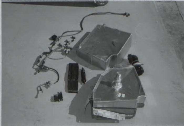
Photo 13) Alternative reservoir , pump , nozzles , solenoid valve , pipes and filter
