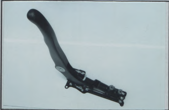
PHOTO N° 15: Parking brake system
