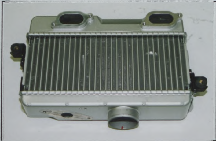
PHOTO N° R) INTERCOOLER DISMOUNTED
