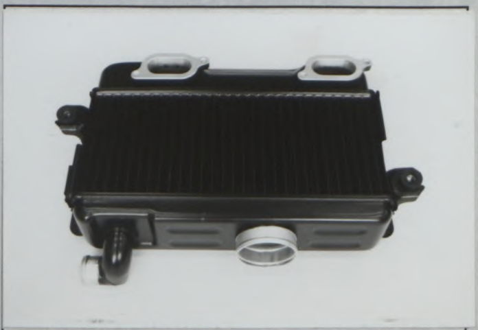
Photo R) Intercooler dismantled
