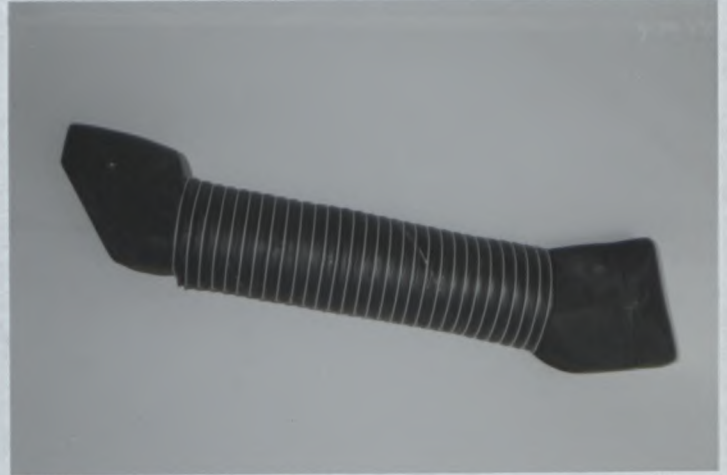
PHOTO N° 2) Brake cooling duct
