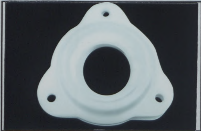
PHOTO N° 21: Steering column bearing
