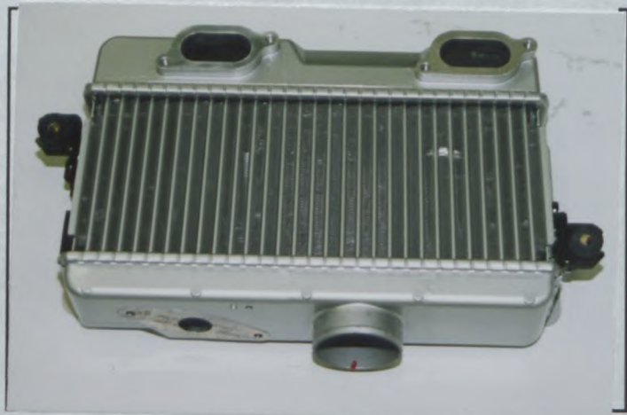
PHOTO N° R) INTERCOOLER DISMOUNTED
