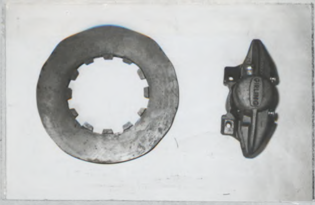
Photo F : Front brake , disc with calliper(s)
