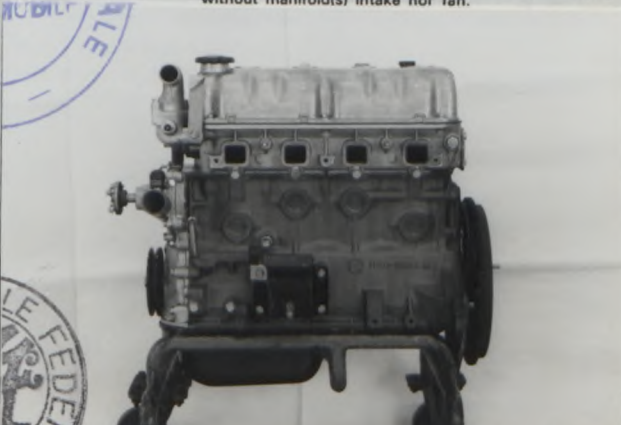
Photo J View of the engine, left side, without accessories, without manifold(s) intake nor fan.
