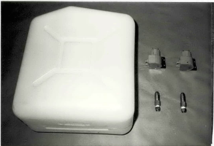
TANK , PUMPS , INJECTORS.
