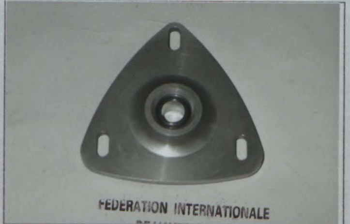
PHOTO No 12 REINFORCED REAR TOP MOUNT
