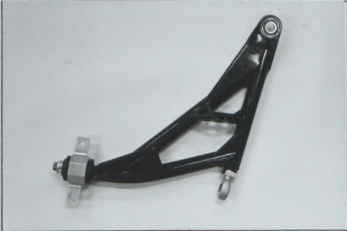
PHOTO No 13 REINFORCED FRONT LOWER ARM
