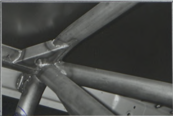
PHOTO No 5 Main hoop to roof
