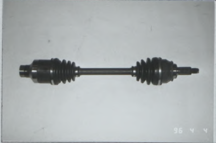
PHOTO No 7 REINFORCED DRIVE SHAFT ( RH )
