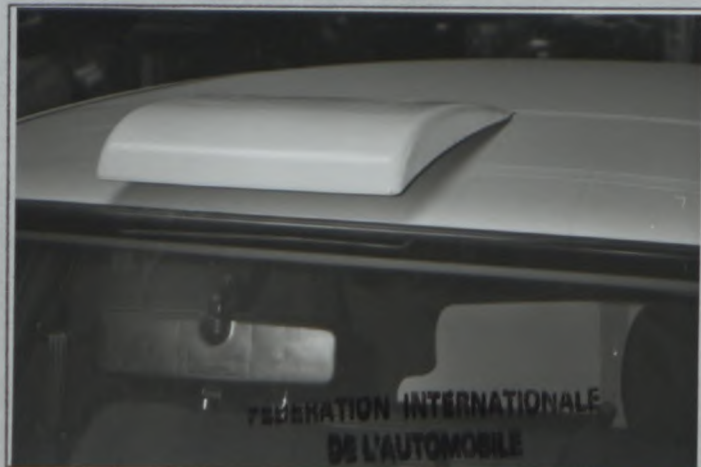
PHOTO No 36 FLAPS FOR VENTILATION
