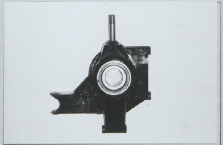
PHOTO No 20 REINFORCED FRONT KNUCKLE
