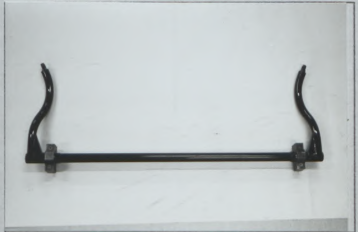
PHOTO No 16 REINFORCED FRONT STABILIZER-BAR
