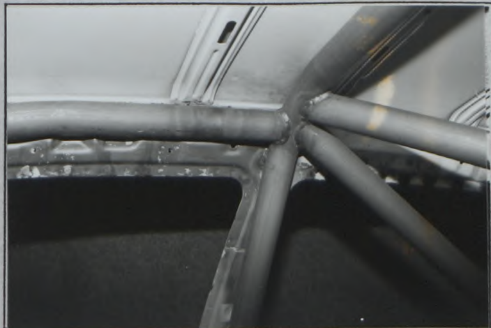
PHOTO No 6. Main/Lateral/Diagonal bar joint
