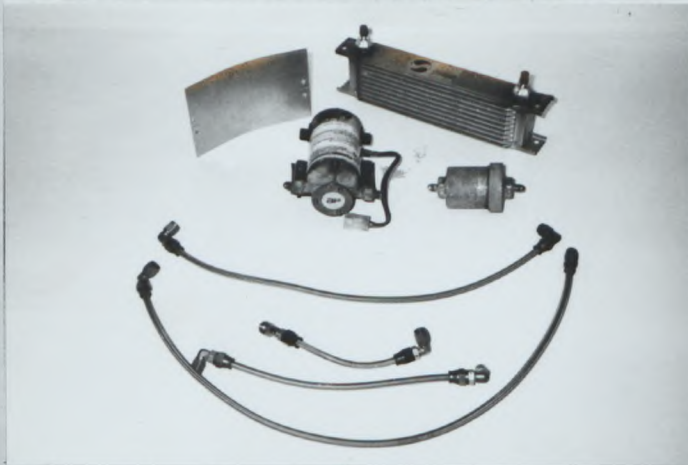
PHOTO No. 1 REAR DIFFERENTIAL COOLING DEVICE WITH ELECTRIC PUMP
