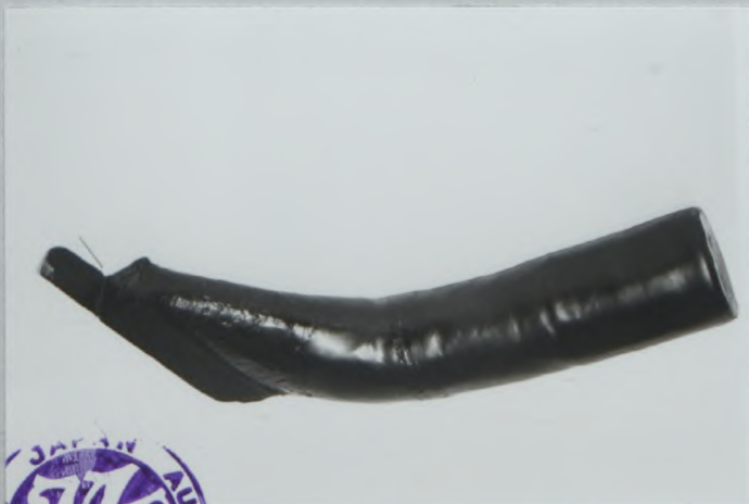
PHOTO No. 5 BRAKE COOLING DUCT.
