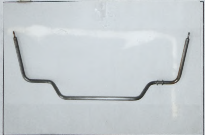
PHOTO No 2. Rear stabirizer bar JA-152 VO-11/11
