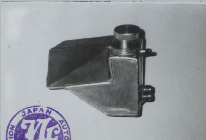
RESERVOIR FOR POWER Photo 11 STEERING & BRAKE COOLING
