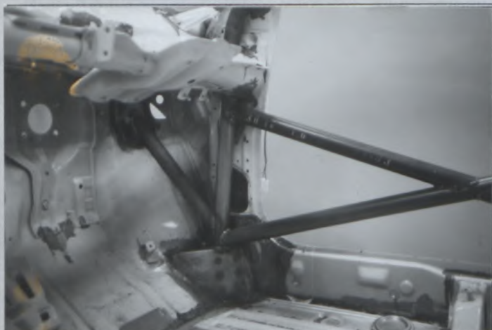
PHOTO No. 1 Lateral bar to floor
