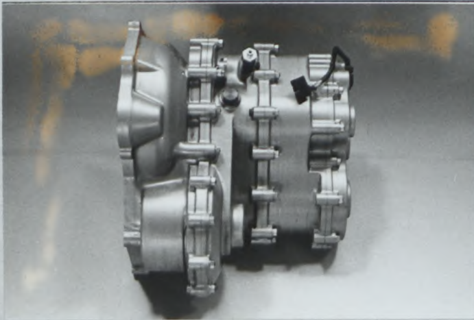
PHOTO No. 1 GEAR BOX.
