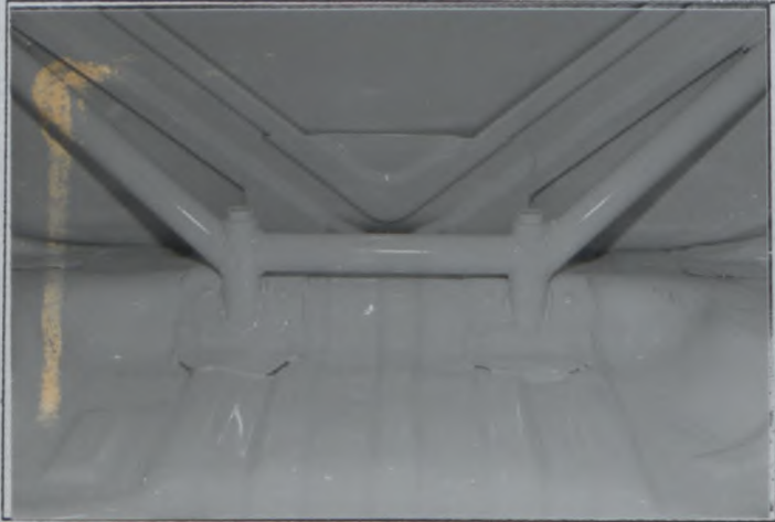
Rear framework to floor, upper
