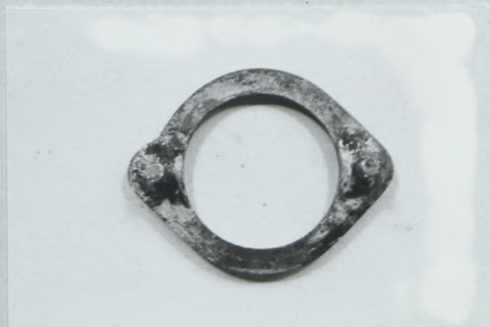
PHOTO No. 8 TOP MOUNT REINFORCEMENT - REAR.
