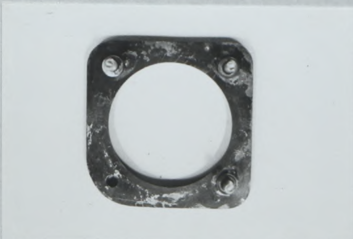
PHOTO No. 9 TOP MOUNT REINFORCEMENT - FRONT.
