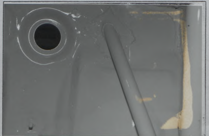
Front turret framework to bulkhead
