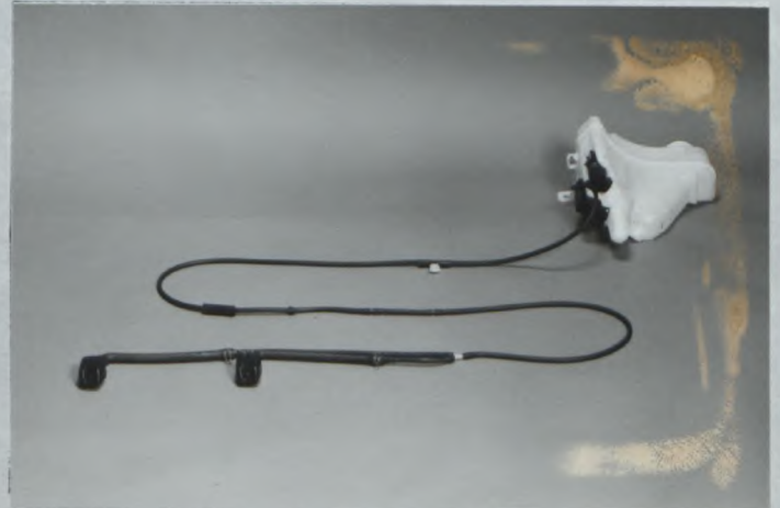
PHOTO No. Z1) WATER SPRAY DEVICE.
