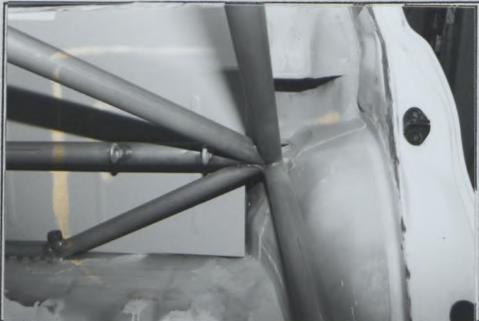
PHOTO No 7. Rear longitudinal/Diagonal to bulkhead
