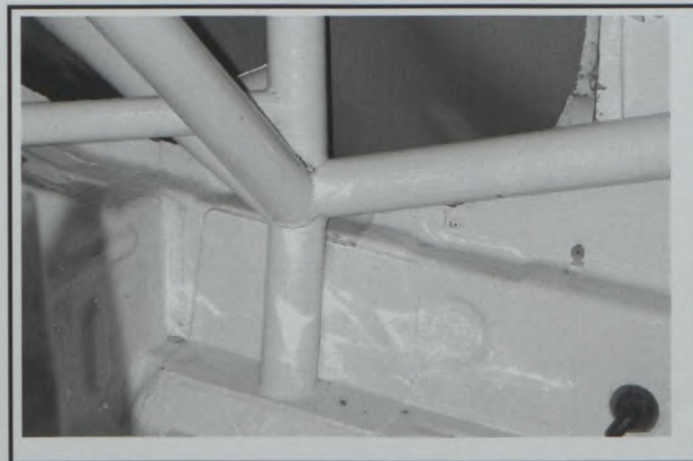
PHOTO N° 10 MAIN HOOP TO FLOOR
