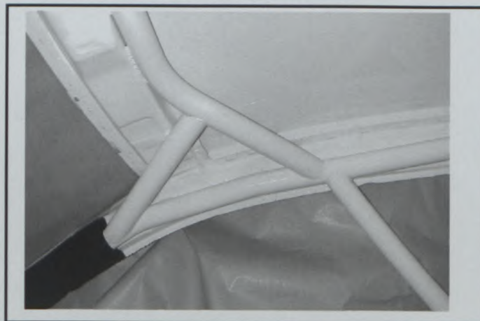
PHOTO N° 3 FRONT HOOP TO ROOF BAR
