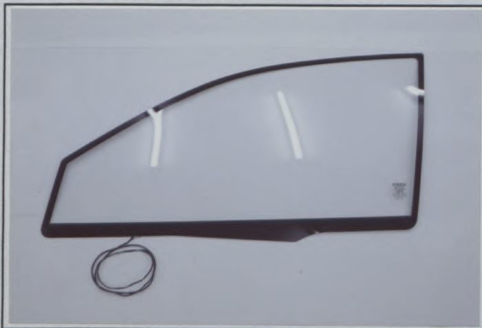
FRONT SIDE WINDOW, WEIGHT = 1.84 kg THICKNESS = 2.4 mm (MIN.)
