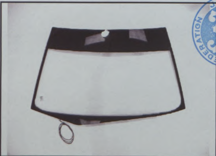
ALTERNATIVE FRONT WINDOW, WEIGHT = 10.22KG, THICKNESS = 3.9MM (MIN)
