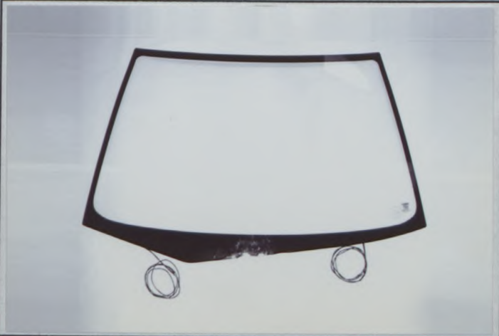
FRONT WINDOW, WEIGHT = 5.95 kg THICKNESS = 2.4 mm (MIN.)
