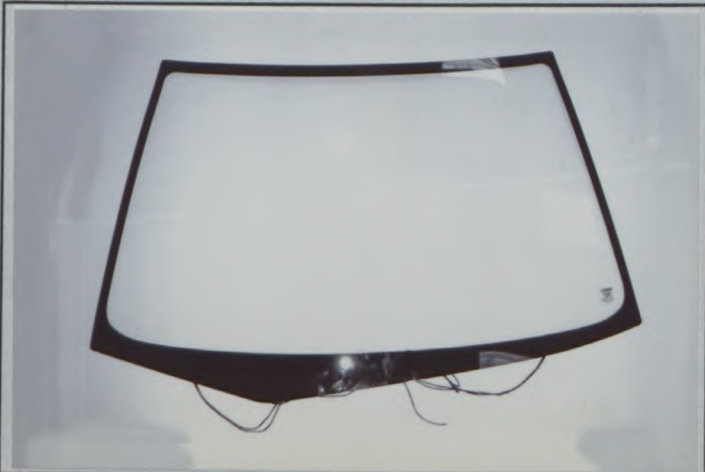
ALTERNATIVE FRONT WINDOW, WEIGHT = 9.2 kg THICKNESS = 3.5 mm (MIN.)
