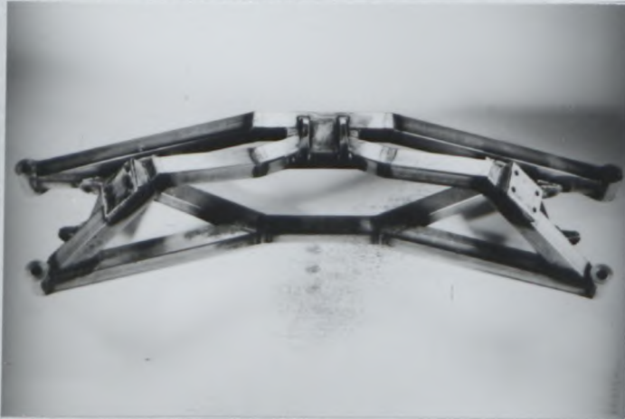
PHOTO No. 7 REAR SUBFRAM
