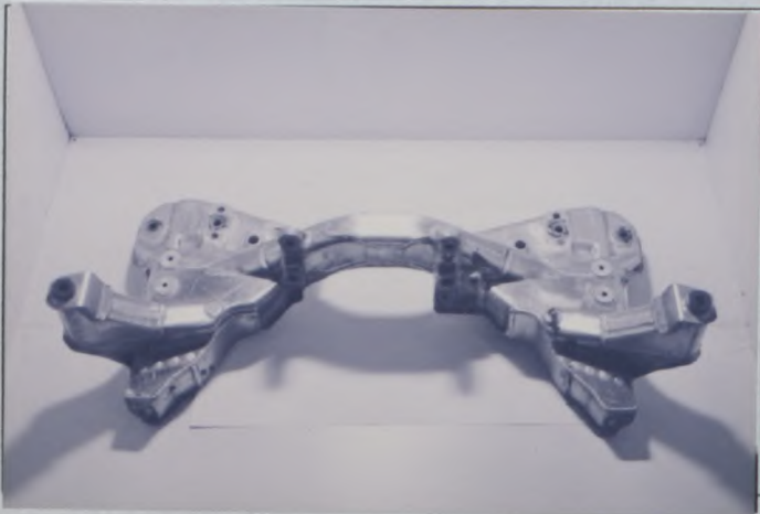
PHOTO No. 55 FRONT SUBFRAME
