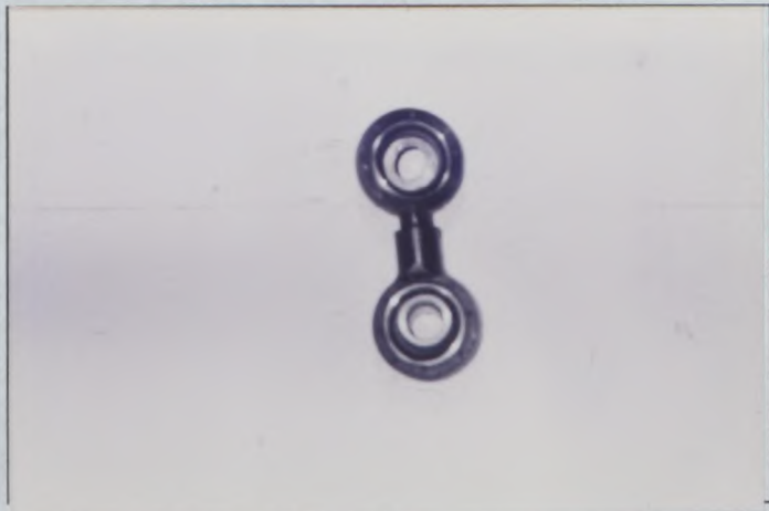
PHOTO No. 36 STABILIZER BAR LINK
