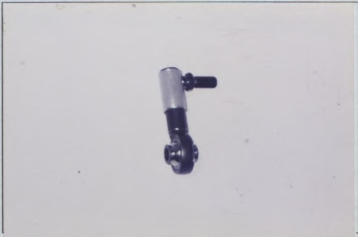
PHOTO No. 36A REINFORCED STABILIZER BAR LINK
