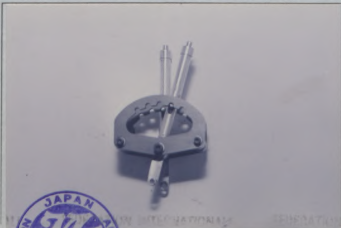
PHOTO No. 34 STABILIZER BAR CONTROL SYSTEM - FRONT
