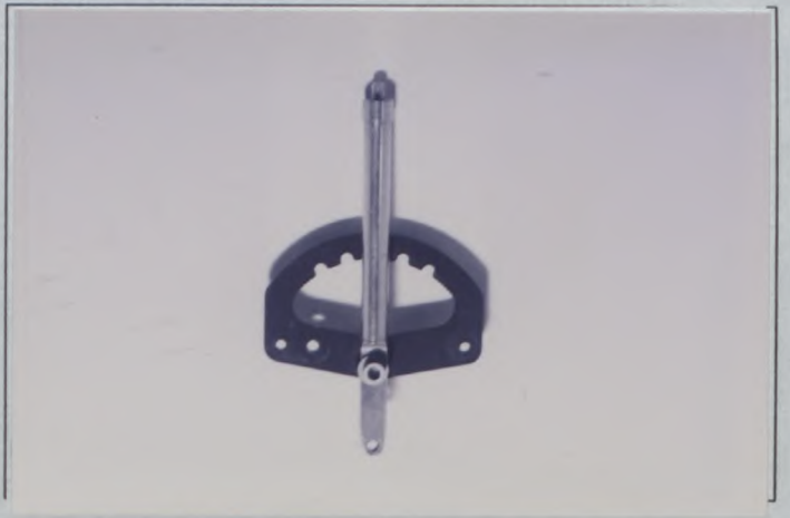
PHOTO No. 33 STABILIZER BAR CONTROL SYSTEM - FRONT
