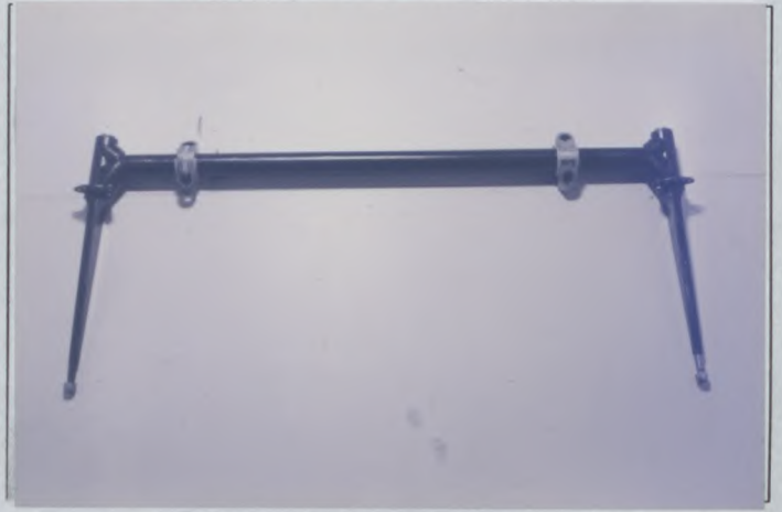
PHOTO No. 31 REAR ADJUSTABLE STABILIZER BAR
