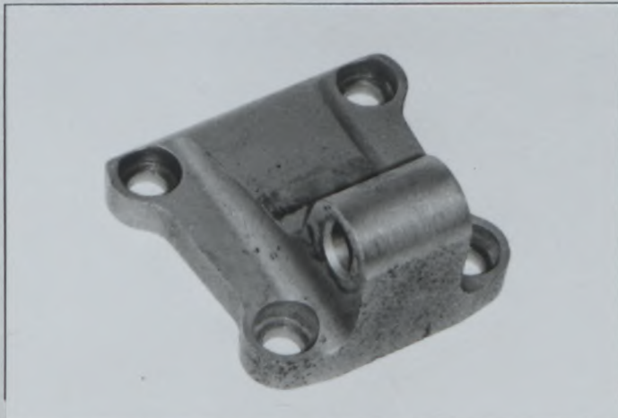
PHOTO No. 6 REAR DIFFERENTIAL MOUNTING BLOCK
