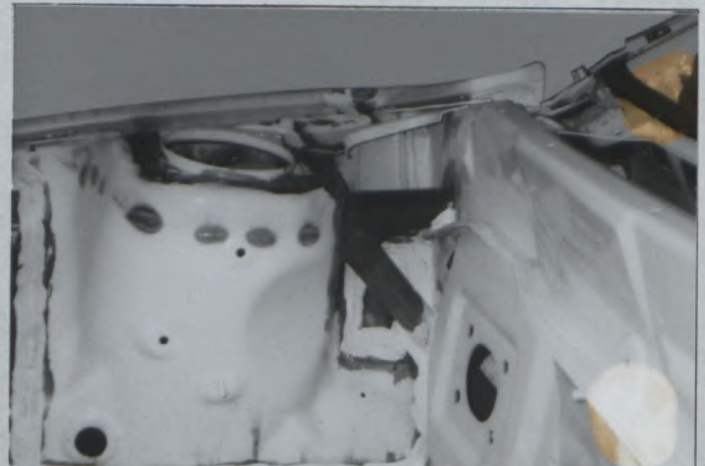
PHOTO No.10 Front framework to turret
