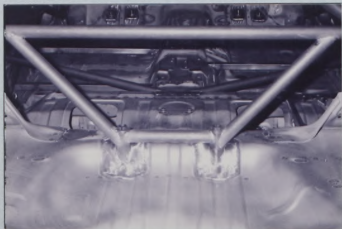
PHOTO No. 3 Rear framework to floor, upper
