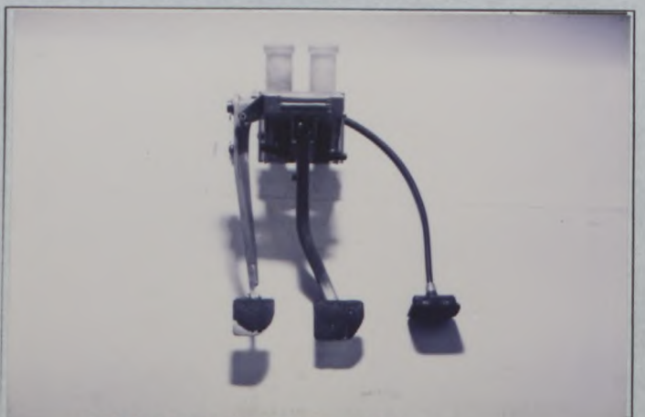
PHOTO No. 82 TWIN BRAKE MASTER CYLINDER
