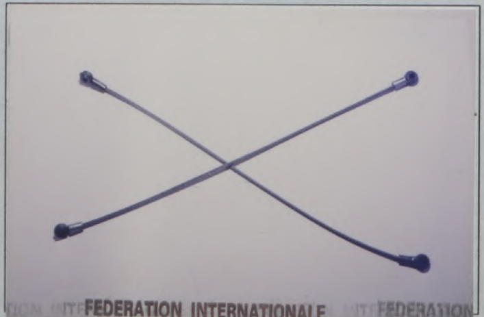
PHOTO No. 58 RESTRAINT STRAP FOR FRONT SUBFRAME
