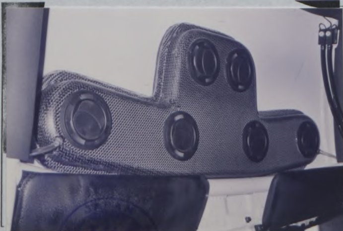
PHOTO No. 99 FLAPS FOR VENTILATION
