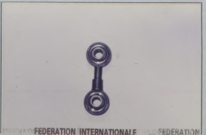
PHOTO No. 35 STABILIZER BAR LINK
