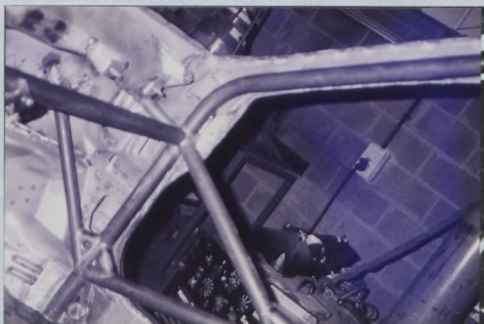
PHOTO No. 8 Lateral bar to A-pillar
