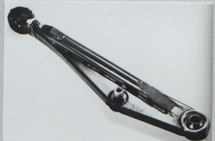
PHOTO No. 6 REAR LOWER LINK
