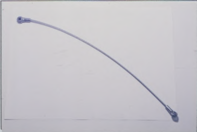
PHOTO No. 59 RESTRAINT STRAP FOR FRONT SUBFRAME
