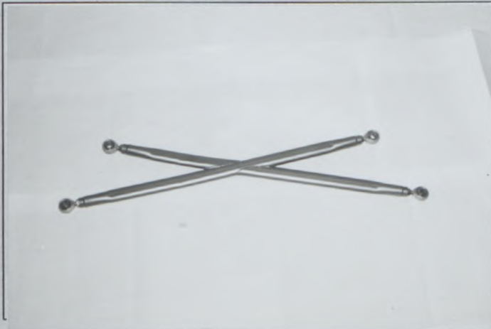
PHOTO No. 61 RESTRAINT STRAP FOR FRONT SUBFRAME
