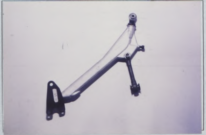
PHOTO No.14A LOWER ARM - FRONT
