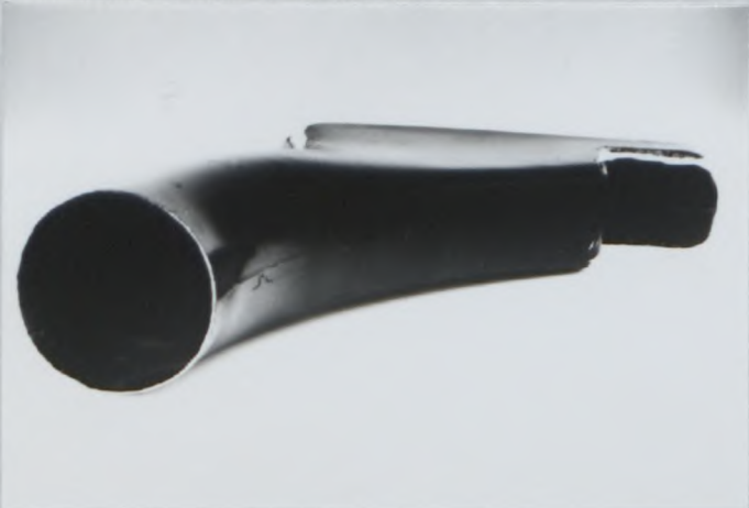
PHOTO No. 9 BRAKE COOLING DUCT
