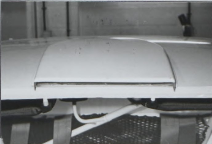
PHOTO No. 97 FLAPS FOR VENTILATION
