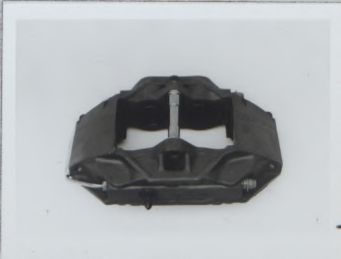
PHOTO V2 FRONT BRAKE CALIPER, TYPE B
