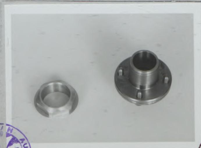
PHOTO U10 CENTRAL WHEEL BOLTING SYSTEM, TYPE A
