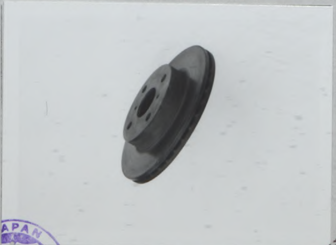
PHOTO V9 FRONT BRAKE DISC, TYPE C
