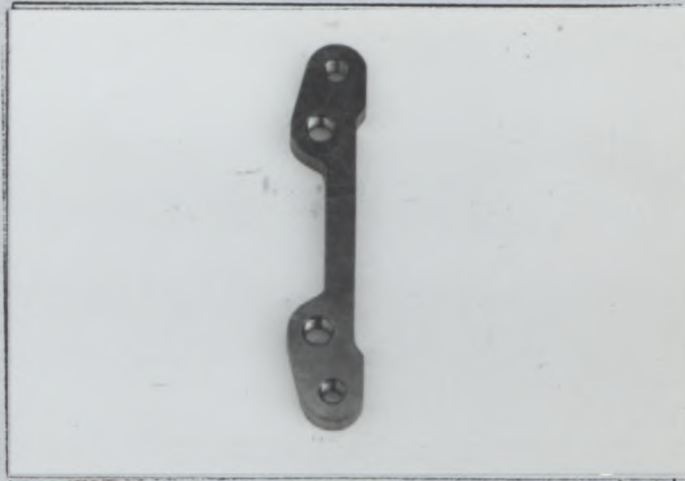
PHOTO U13 CALIPER MOUNTING BRACKET, TYPE B
