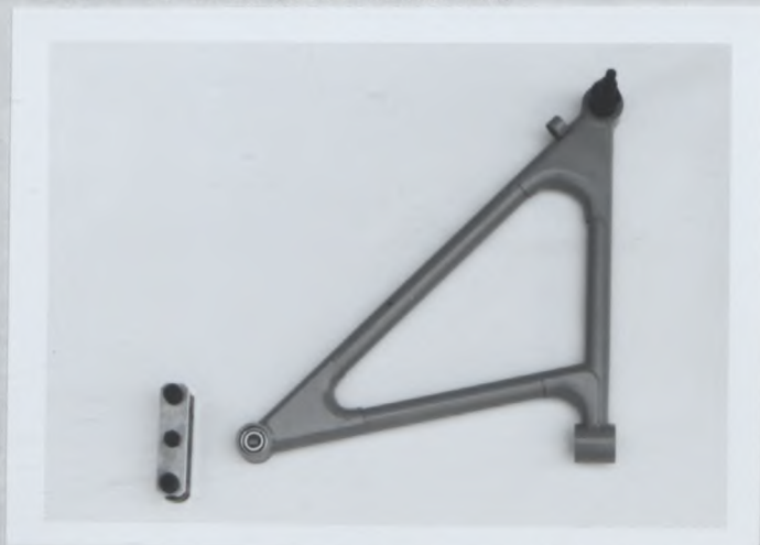
PHOTO T1 REINFORCED LOWER ARM
