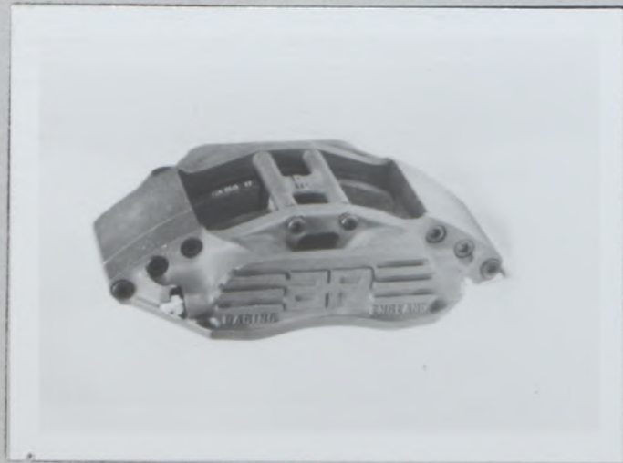
PHOTO V1 FRONT BRAKE CALIPER, TYPE A
