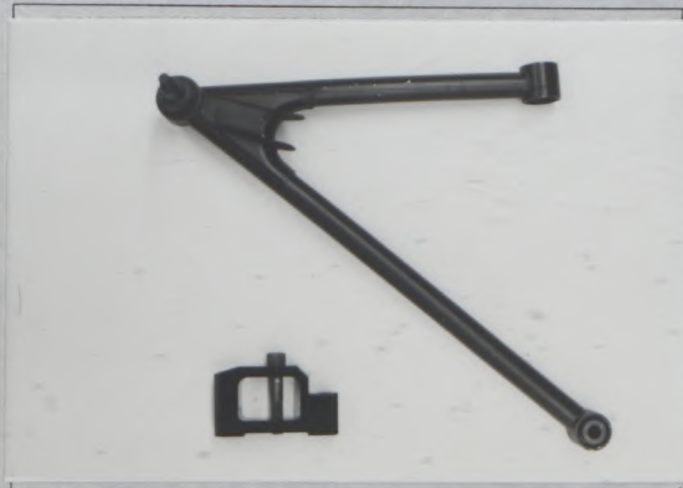
PHOTO T1 REINFORCED LOWER ARM
