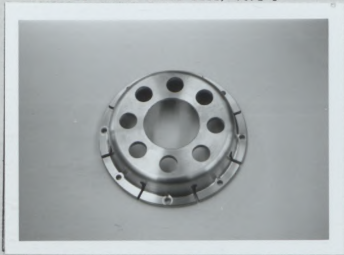
PHOTO V11 FRONT BRAKE BELL, TYPE B
