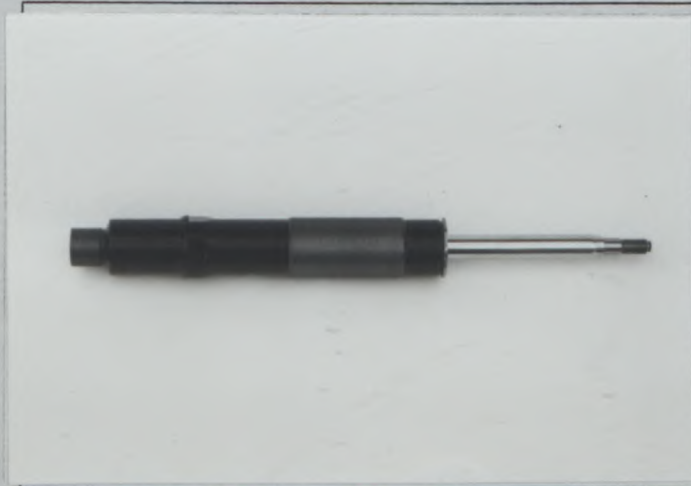
PHOTO U8 REINFORCED REAR STRUT, TYPE B
