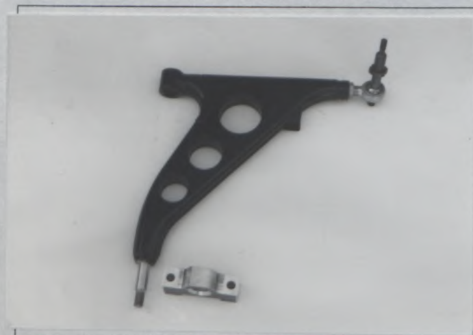
PHOTO T3 REINFORCED LOWER ARM, TYPE B
