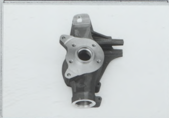
PHOTO U6 REINFORCED REAR AXLE CARRIER, TYPE B
