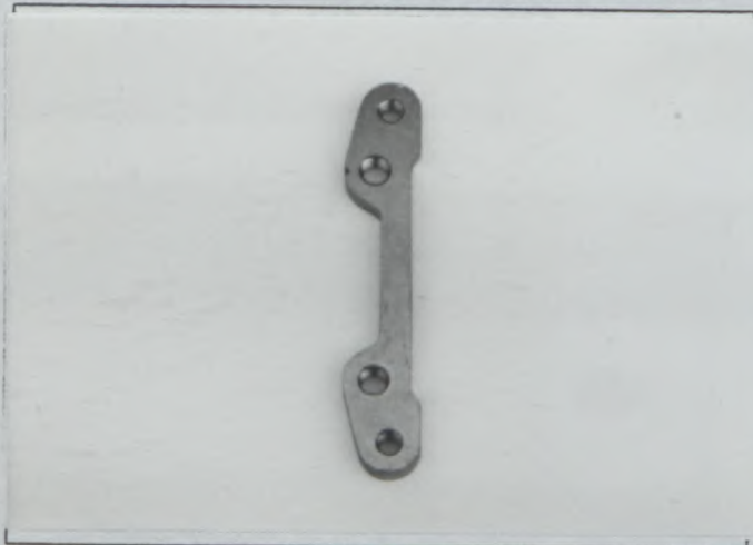
PHOTO T13 CALIPER MOUNTING BRACKET, TYPE B
