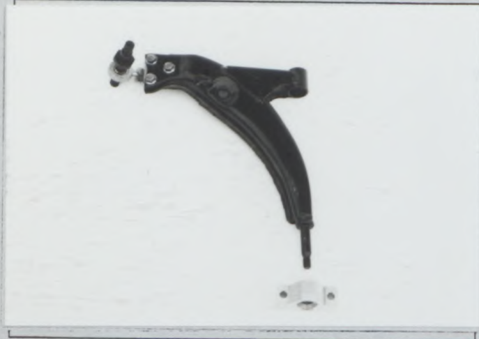
PHOTO T1 REINFORCED LOWER ARM, TYPE A
