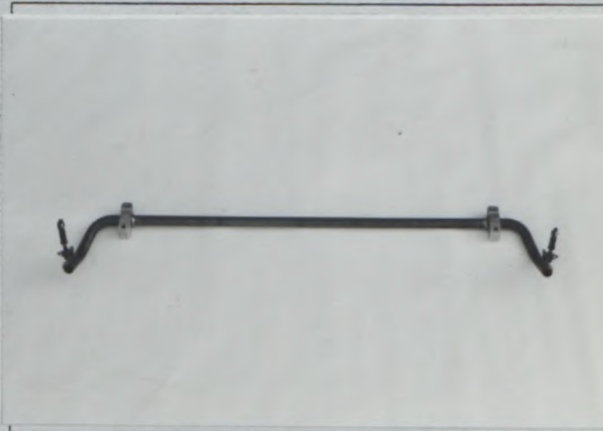
PHOTO U9 ADJUSTABLE STABILIZER WITH LINKAGE
