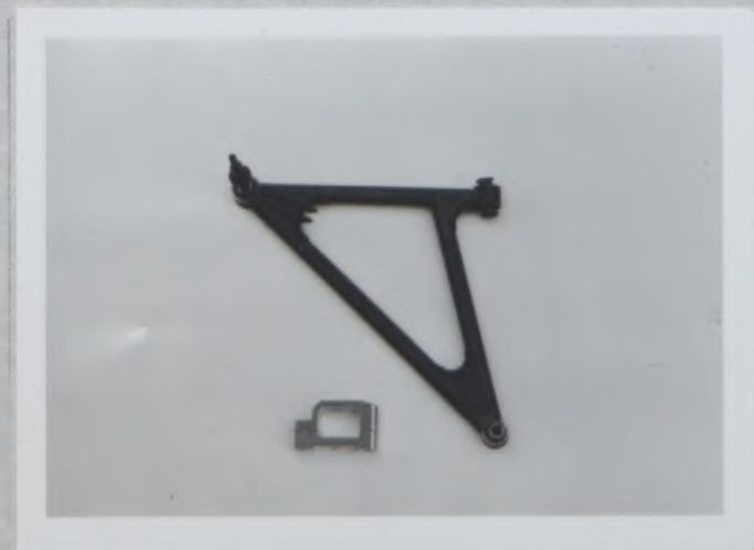
PHOTO T1 REINFORCED LOWER ARM
