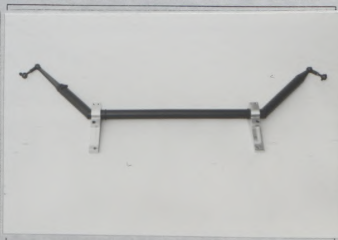
PHOTO T2 ADJUSTABLE STABILIZER WITH LINKAGE
