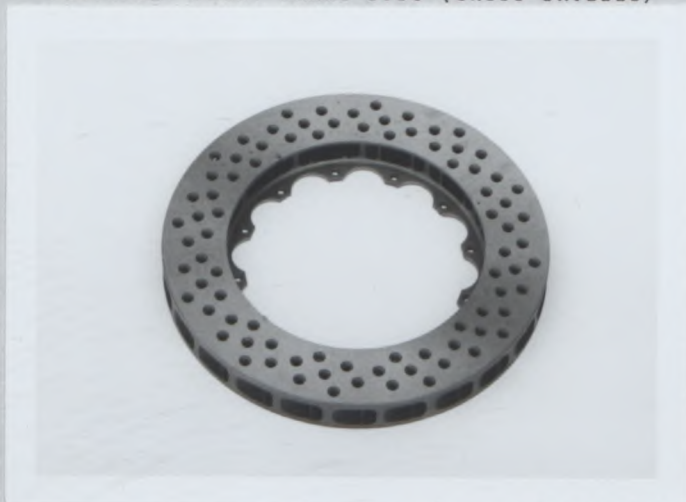
PHOTO V2 FRONT BRAKE DISC (CROSS-DRILLED)
