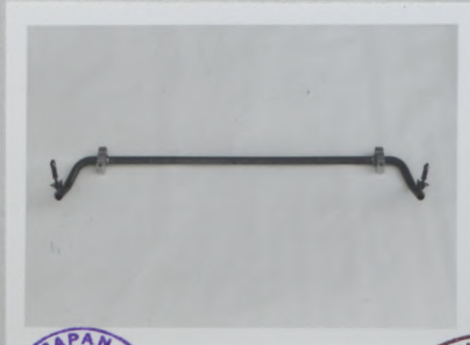
PHOTO U ADJUSTABLE STABILIZER WITH LINKAGE
