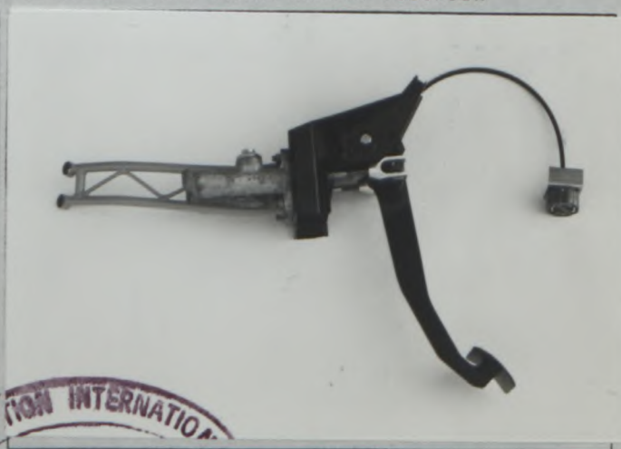
PHOTO Z3 TWIN BRAKE MASTER CYLINDER
