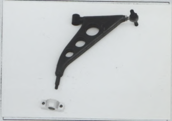
PHOTO T2 REINFORCED LOWER ARM, TYPE B
