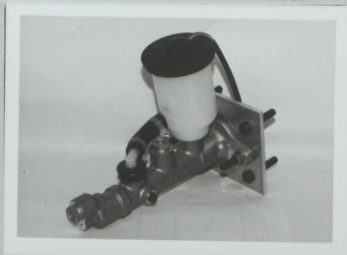
PHOTO Z1 TANDEM BRAKE MASTER CYLINDER
