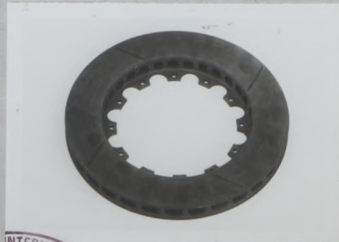
PHOTO V1 FRONT BRAKE DISC (GROOVED)
