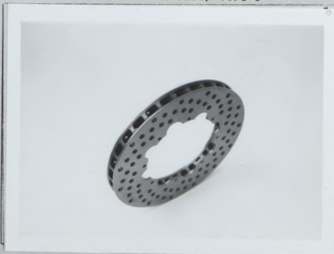
PHOTO V8 FRONT BRAKE DISC, TYPE B
