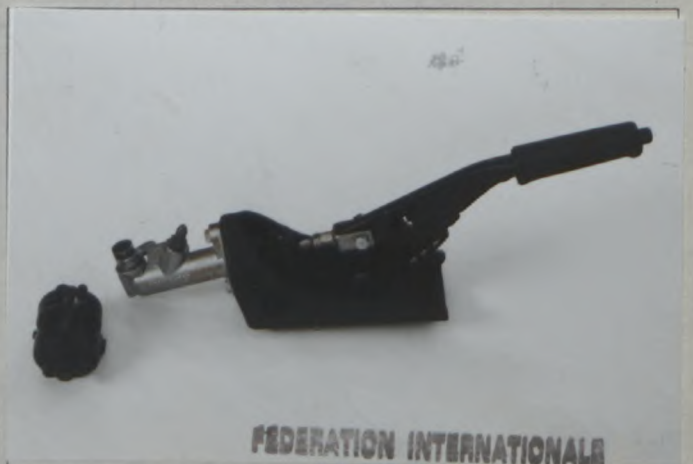
PHOTO No. 6 (PARKING BRAKE)
