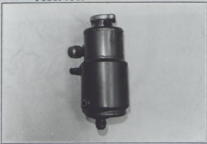
FB) Water cooled steering fluid reservoir
