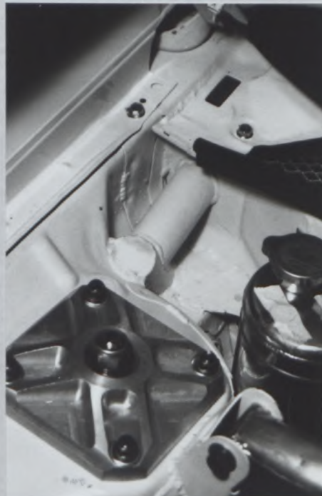
Front reinforcement to front strut tower
