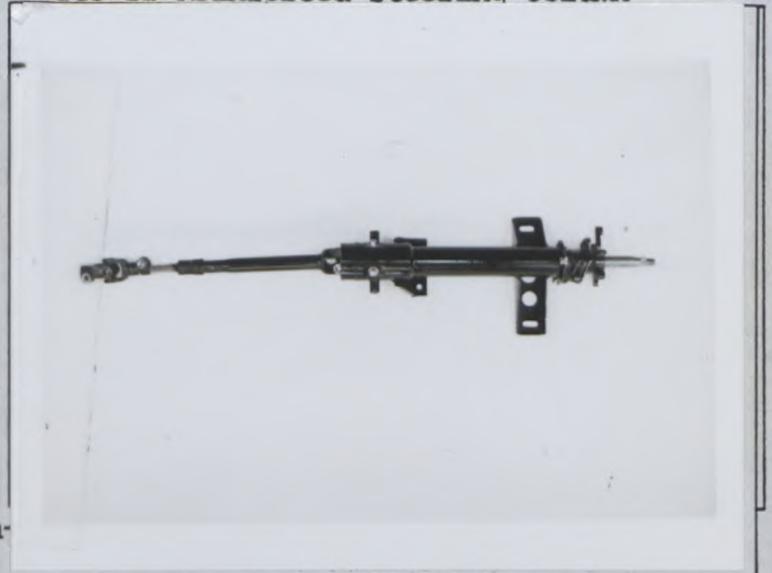
Photo Z2 Reinforced steering column
