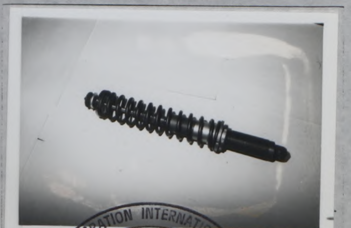
Alternative position of rear spring Photo U5 and shock absorber
