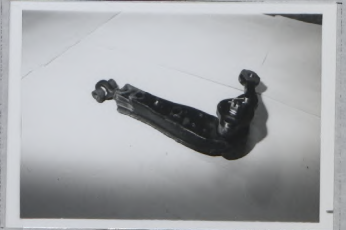
Reinforced front lower arm Photo T2 (Type B)
