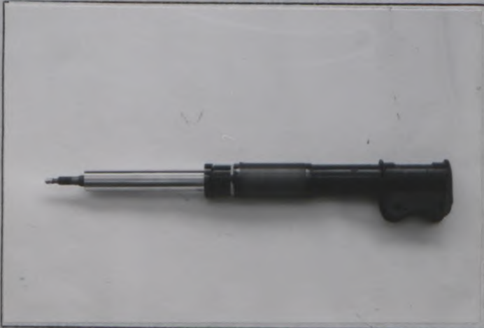
Photo T3 Reinforced front strut
