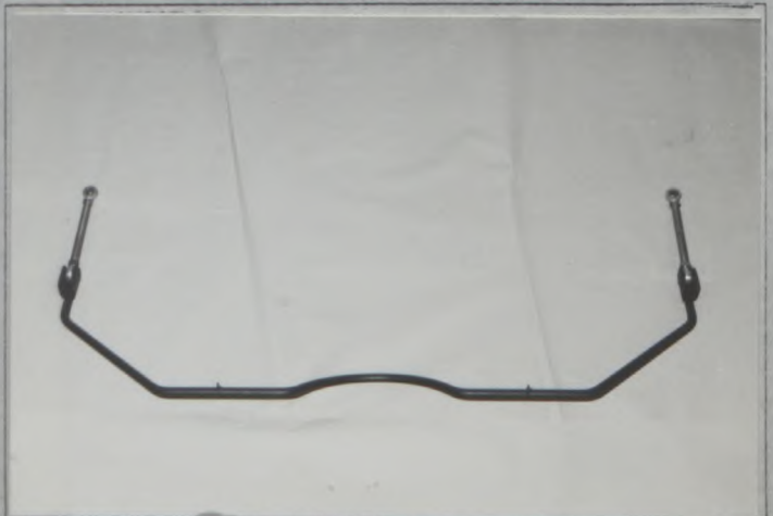
Photo U2 Rear stabilizer with linkage
