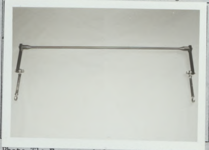
Photo T1: Front stabilizer with linkage
