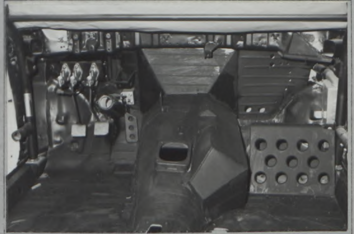
Photo Z8 Modified gearbox tunnel
