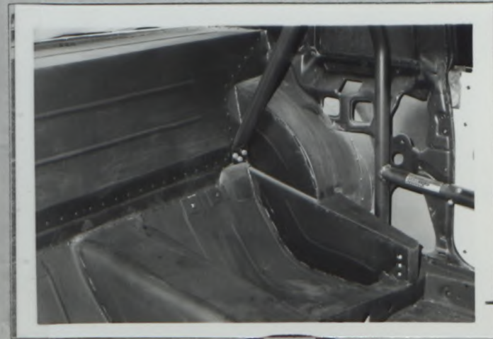
Photo Z2 Location of upper control arm and modified inner wheel arch
