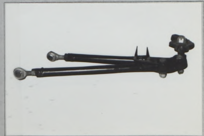
Alternative track control arm and caster-rod
