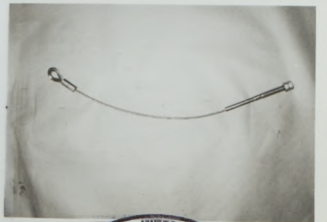
Photo Z5 Suspension limiter
