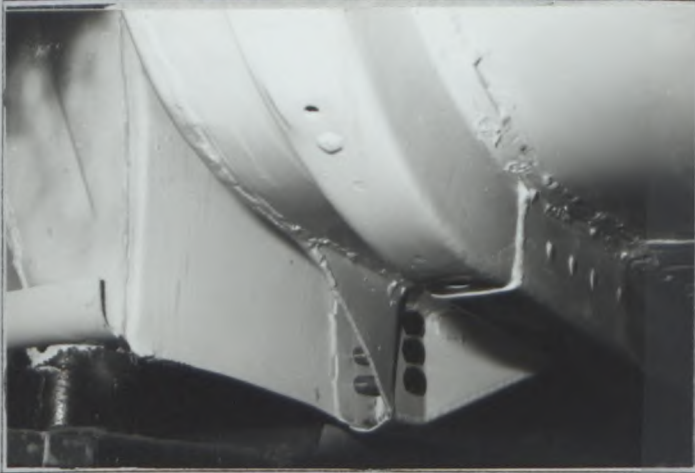
Photo Z5 Location of rear shock absorber turret
