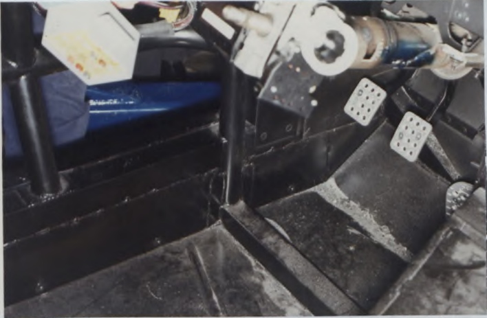
PHOTO No LEFT FRONT ROLLBAR WELDED TO FRAME
