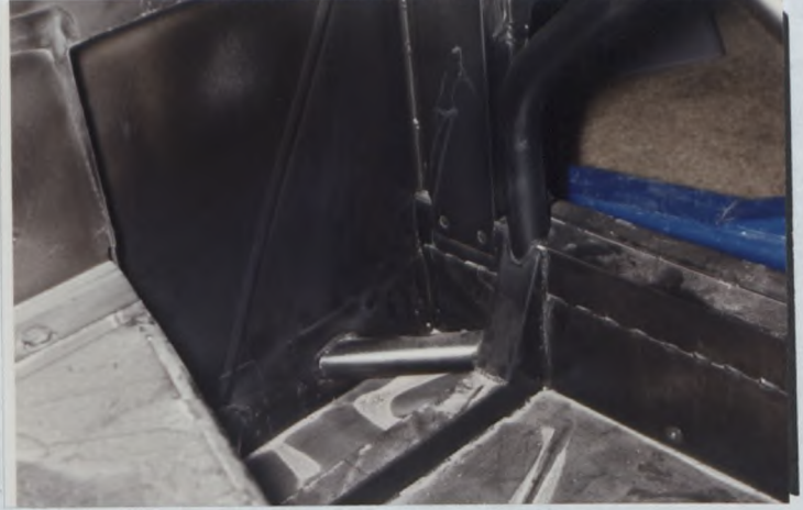
PHOTO No RIGHT FRONT ROLLBAR WELDED TO FRAME
