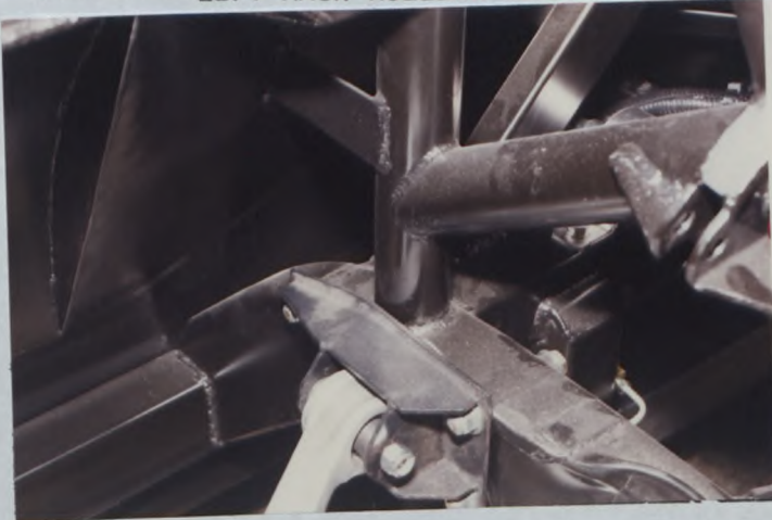
PHOTO No LEFT MAIN ROLLBAR WELDED TO FRAME
