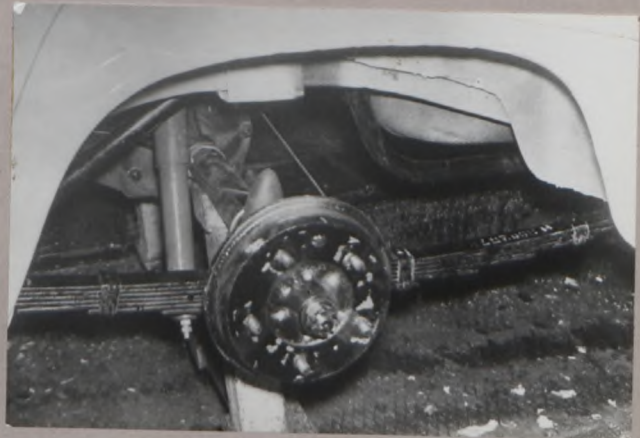
Rear suspension system showing rubber buffer limiting jounce travel and shock absorber limiting rebound travel.
