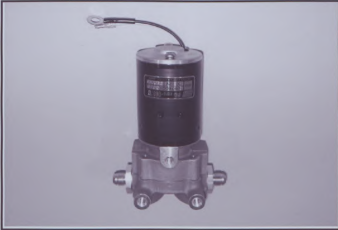
PHOTO N° 6.3 : Gearbox oil pump
