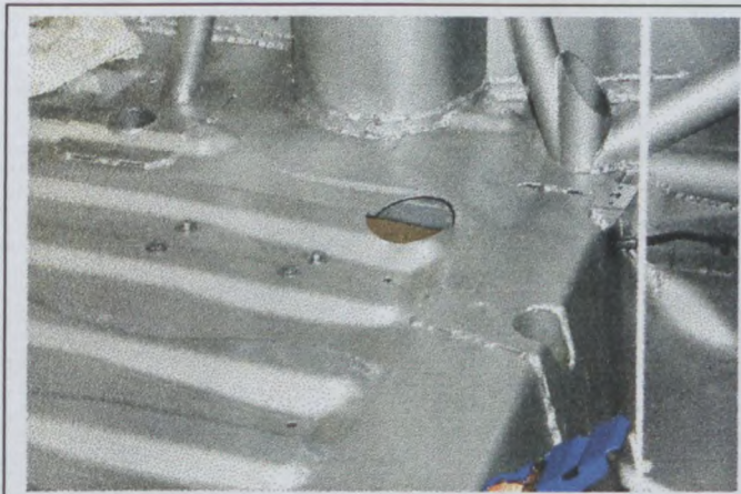
8 / Perçage communication reservoir sup /reservoir inf
