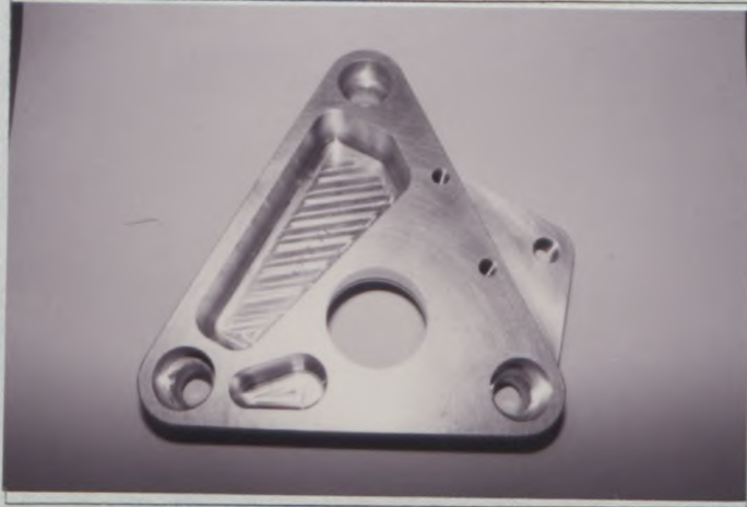
PHOTO No. 1 (FRONT STRUT UPPER MOUNTING)
