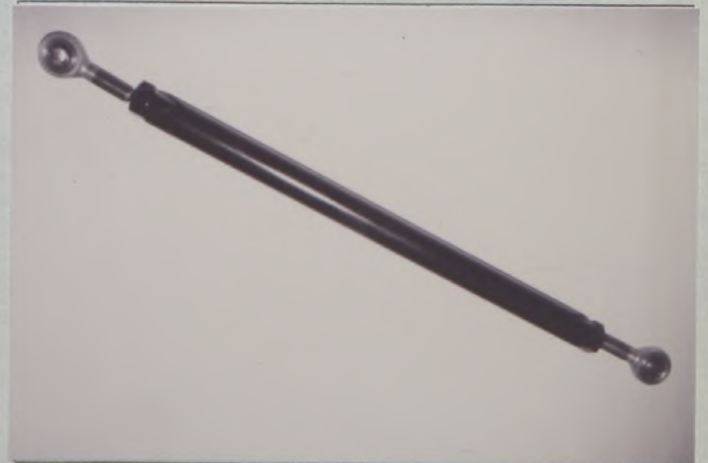
PHOTO No. 4 (REAR TRANSVERSE LINK)
