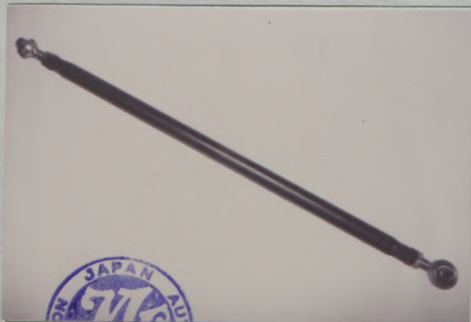
PHOTO No. 5 (REAR TRAILING LINK)
