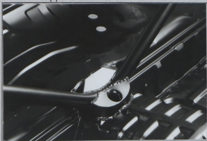
Lateral support to floor
