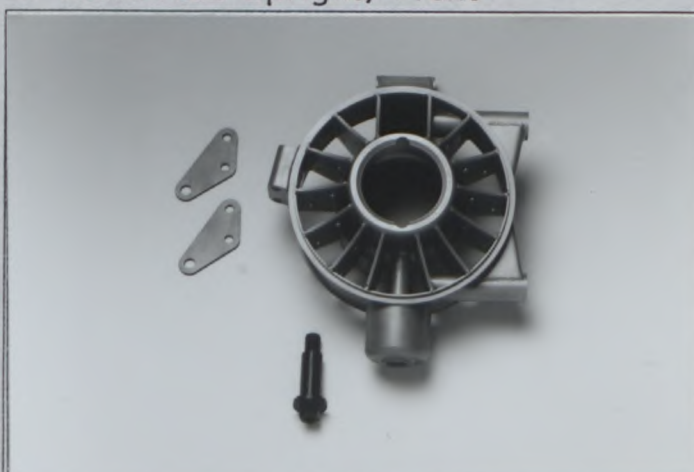
4. Reinforced Upright, Front
