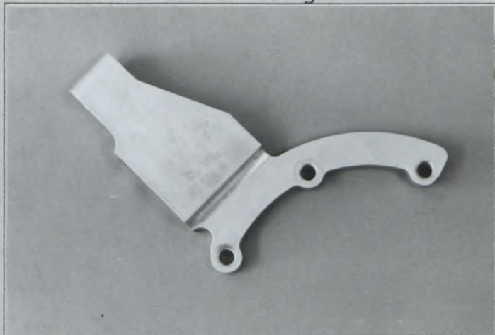
S2 Reinforced brace for gear - box
