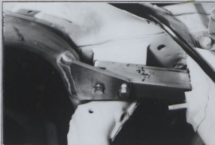
Front support to pillar
