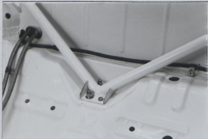
Lateral support to rear floor
