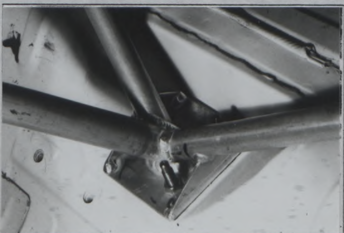
Rear diagonal to floor
