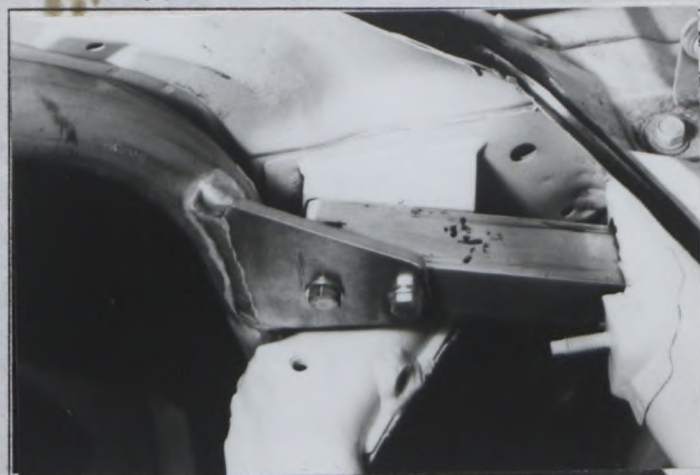
Front support to pillar
