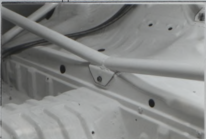
Lateral support to floor
