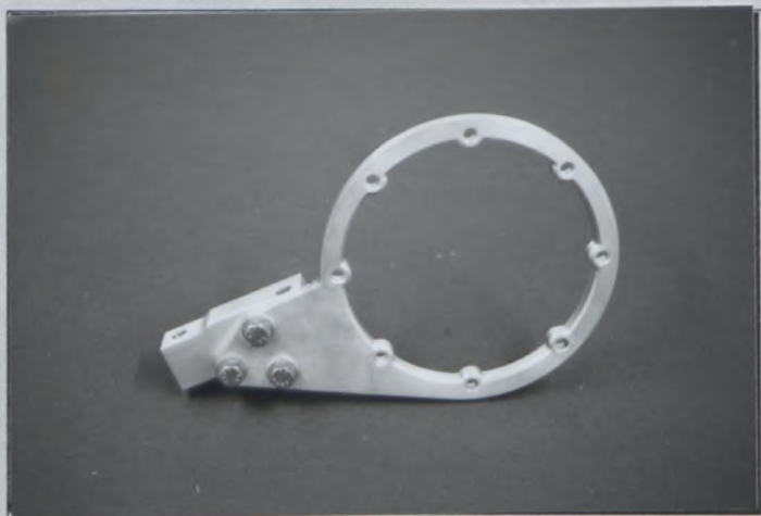
S1 Reinforced brace for gear-box
