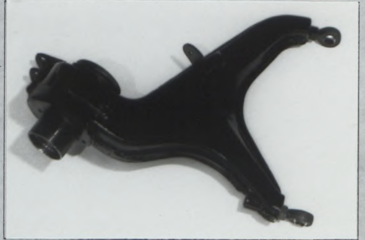
Photo U1 Reinforced rear trailing arm (TypeA)
