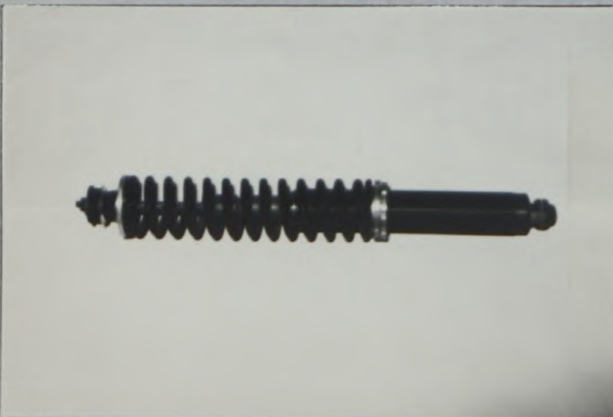
Alternative position of rear Photo U1 spring on shock absorber
