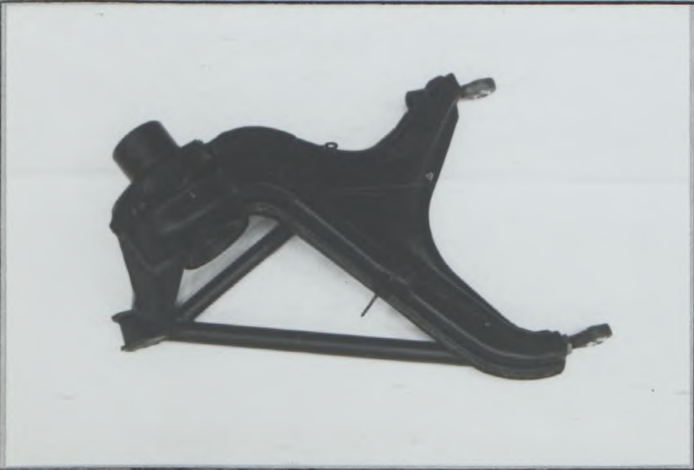
Photo U2 Reinforced rear trailing arm (TypeB)
