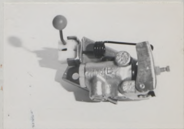
proportionong front rear valve /hydraulic/
