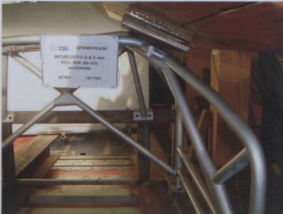
FRONT ROLL BAR STATIC TEST AFTER
