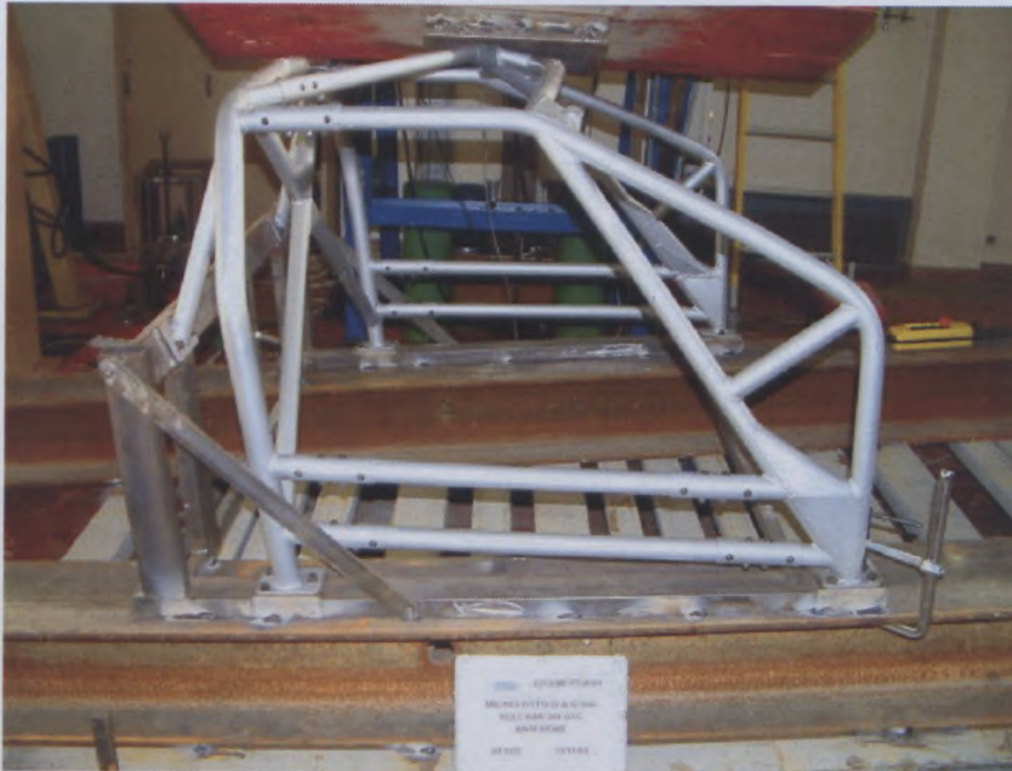
FRONT ROLL BAR STATIC TEST AFTER
