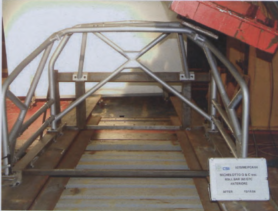
FRONT ROLL BAR STATIC TEST AFTER
