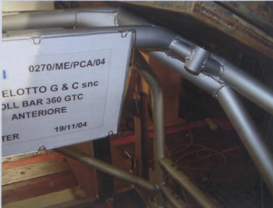
FRONT ROLL BAR STATIC TEST AFTER
