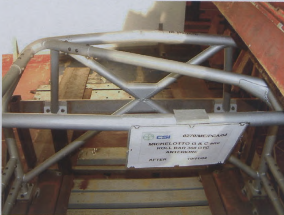
FRONT ROLL BAR STATIC TEST AFTER
