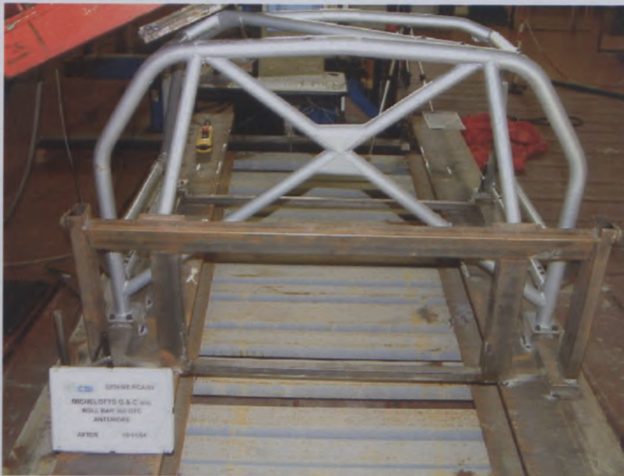
FRONT ROLL BAR STATIC TEST AFTER
