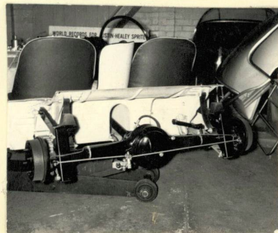
Rear axle complete (without wheels).
