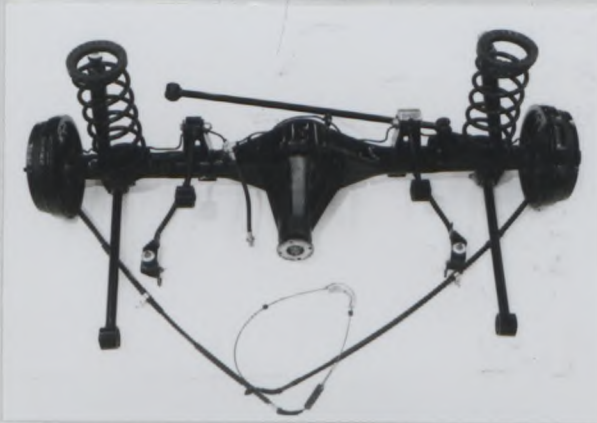
Photo E Complete rear wheels assy removed from car
