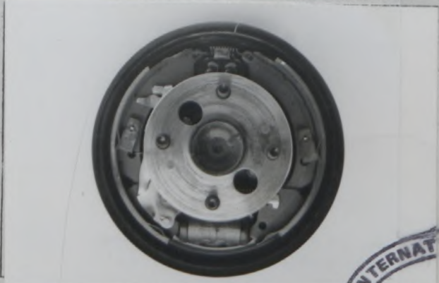
Photo G リアブレーキ、ドラムを除去し、XXXXXXXXXXXXXXXXXXXX Rear brake, drum removed. XXXXXXXXXXXXXXXXXXXXXXX
