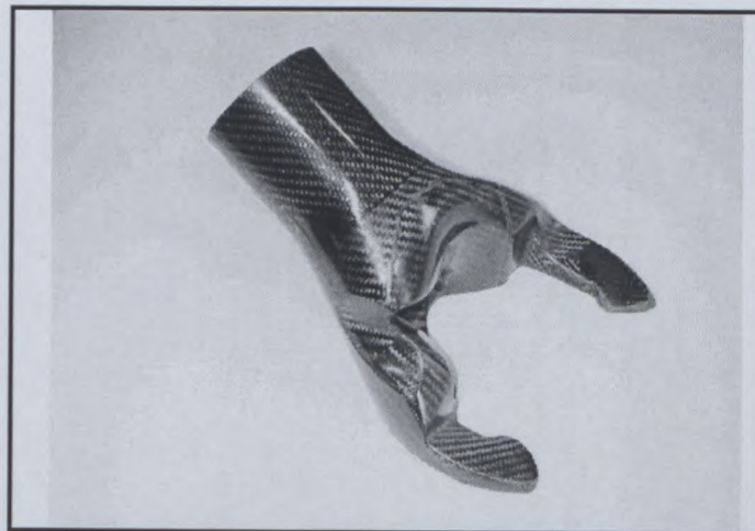
PHOTO N° 32 Brake cooling duct brake side
