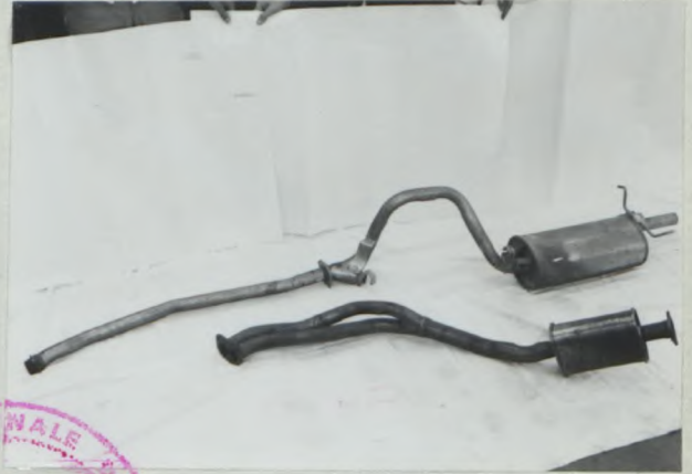
Photo U Exhaust piping with muffler
