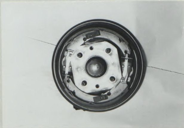
Photo F Front brake, drum removed
