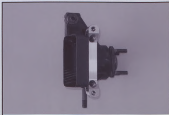
PHOTON° 8.4 : Front brake cooling duct mounted to knuckle
