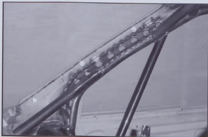
PHOTO N° 3 [NEW] Front hoop to pillar
