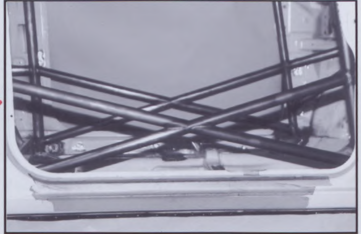
PHOTO N° 14 [OLD] Door cross section
