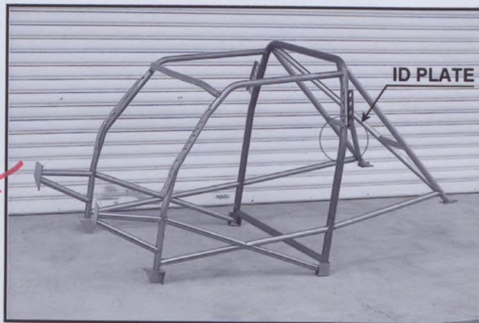
PHOTO N° 2 [OLD] Complete structure of roll cage
