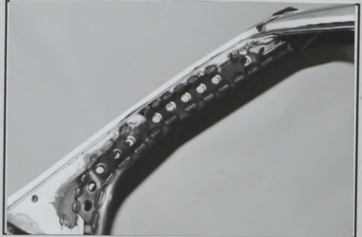
PHOTO N° 1 Front hoop to pillar
