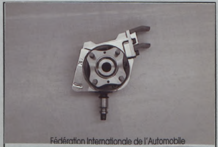
PHOTO N° 30 REINFORCED FRONT KNUCKLE A
