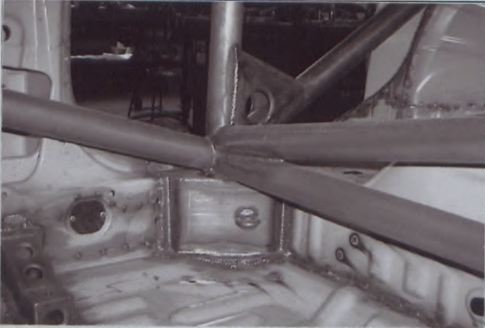
PHOTO N° 6 MAIN HOOP TO FLOOR
