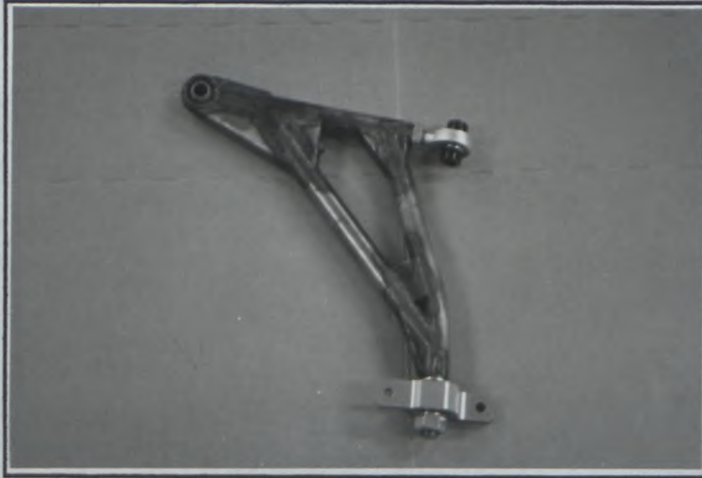
PHOTO N° 19 REINFORCED FRONT LOWER ARM B
