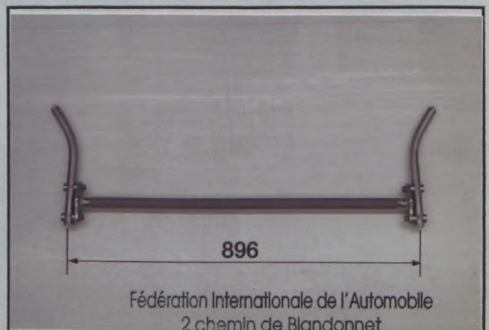
PHOTO N° 24 FRONT STABILIZER-BAR A
