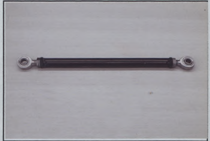
PHOTO N° 20 REINFORCED REAR TRAILING ARM A
