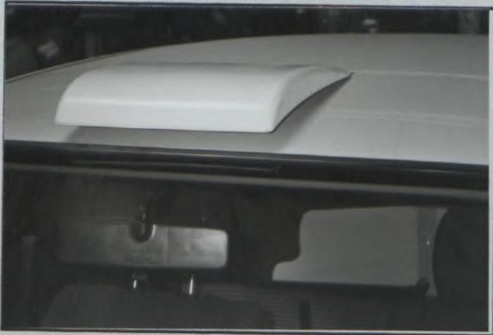
PHOTO N° 57 FLAPS FOR VENTILATION
