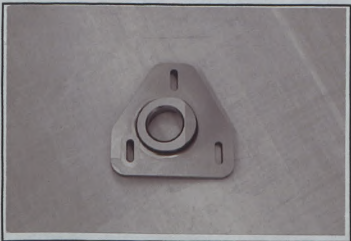
PHOTO N° 15 REINFORCED FRONT TOP MOUNT A
