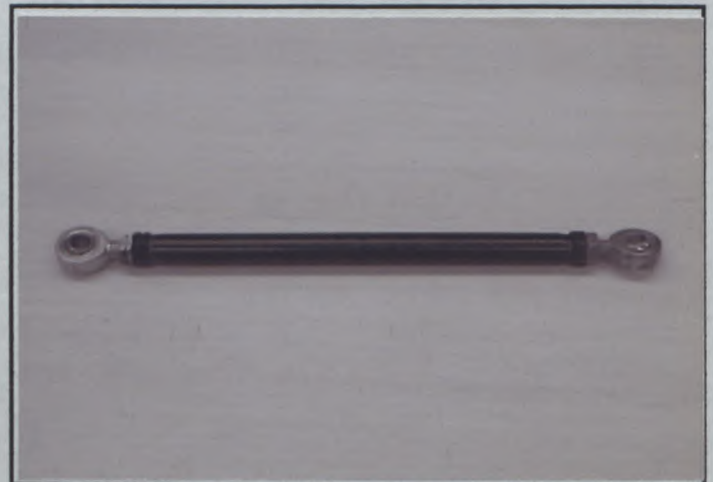
PHOTO N° 22 REINFORCED REAR CONTROL ROD A
