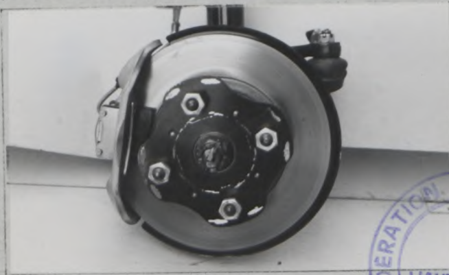
F, Front brake, disc with caliper(s)
