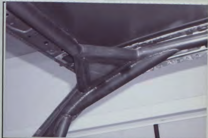
PHOTO N° 9 FRONT LATERAL TO ROOF (RIGHT)
