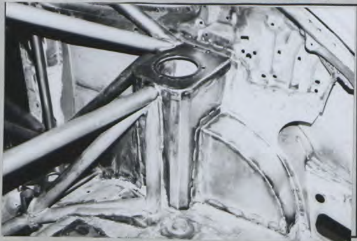
PHOTO N° 14 REAR SUPPORT TO TURRET (RIGHT)
