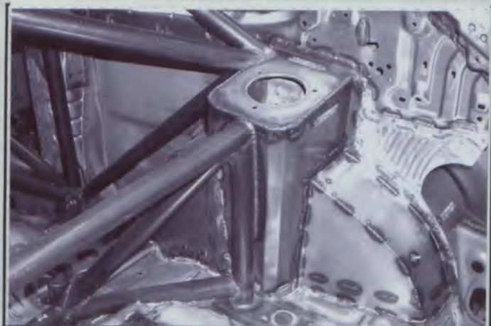
PHOTO N° 12 REAR SUPPORT TO TURRET (RIGHT)
