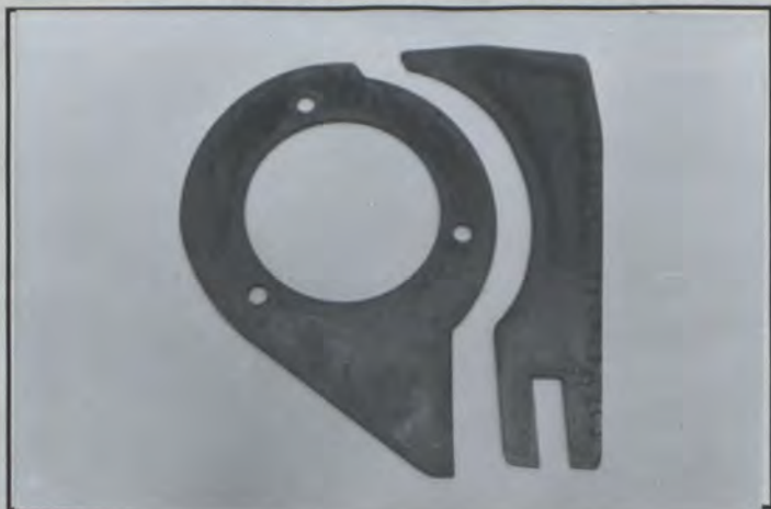
PHOTO N° 1 : Front wheel arch dismantled parts
