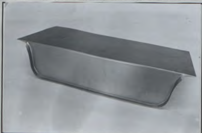
PHOTO N° 9 : Spare wheel dismantled compartment
