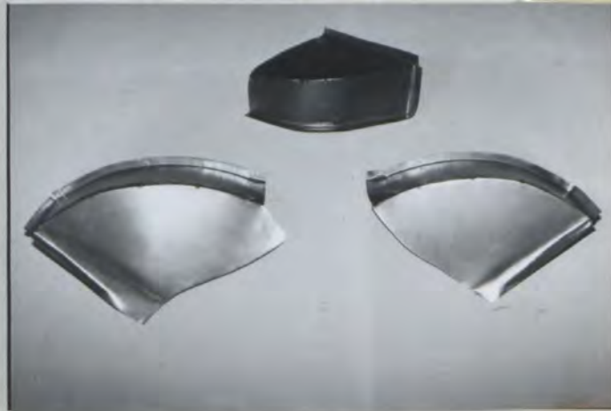
PHOTO N° 4 : Rear wheel arch dismantled parts
