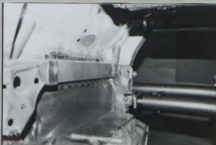
PHOTO N° 12 : Mounted cross member
