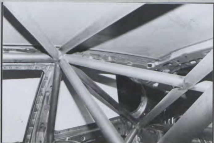
PHOTO N° 8 MAIN HOOP TO ROOF (RIGHT)
