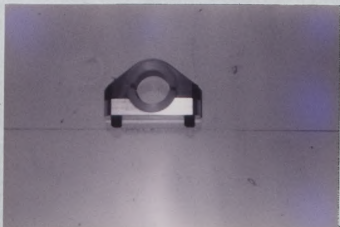
PHOTO No. 44 STABILIZER BAR BRACKET
