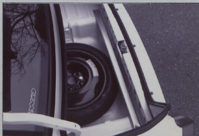
REAR END OF THE CHASSIS RAIL
