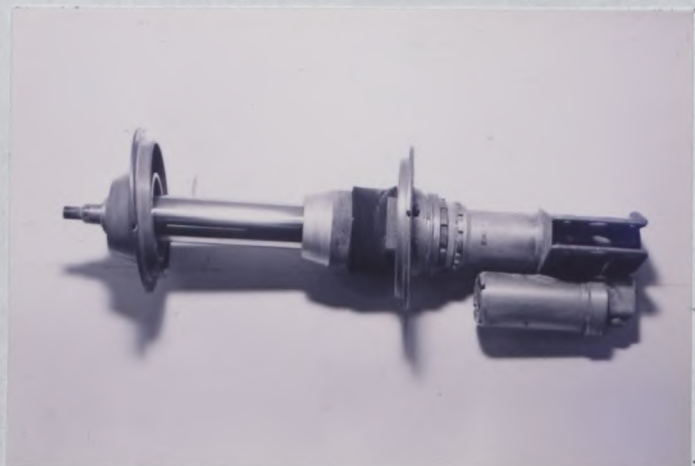
PHOTO No. 32 FRONT DAMPER
