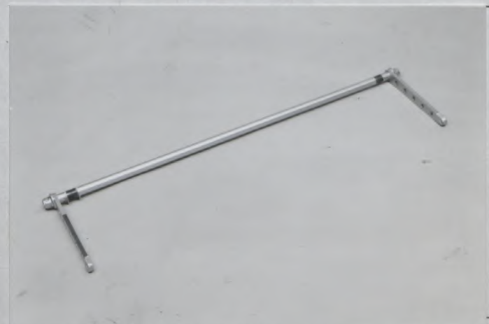
PHOTO No. 40 REAR STABILIZER BAR
