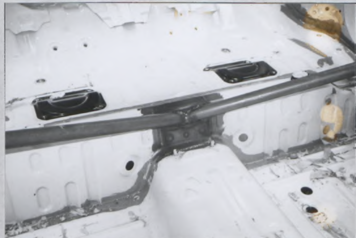
PHOTO No. 8 Central framework to floor
