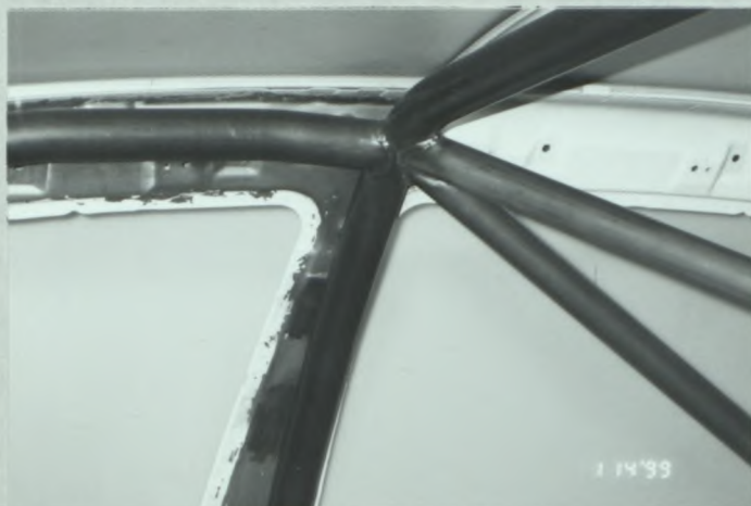
PHOTO N° 6 MAIN / LATERAL / DIAGONAL BAR JOINT
