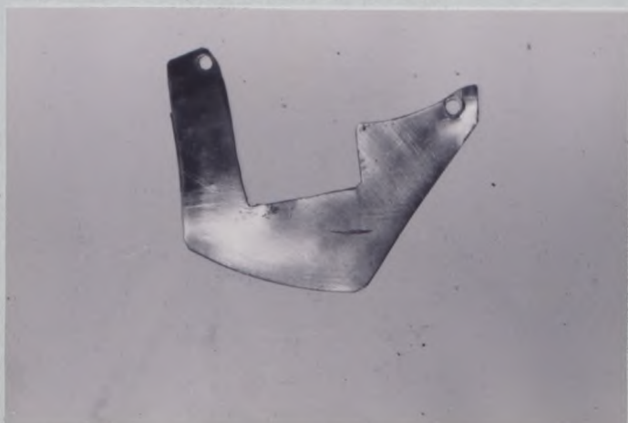
PHOTO No. 87 PROTECTION SHIELD FOR DISC
