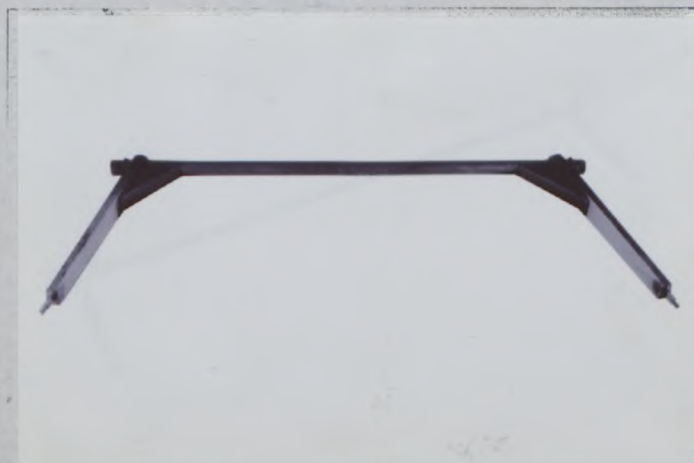
PHOTO No. 39 REAR STABILIZER BAR
