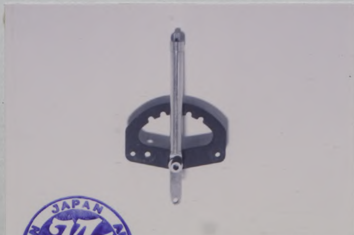
PHOTO No. 41 STABILIZER BAR CONTROL SYSTEM
