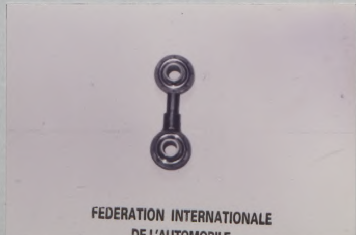
PHOTO No. 42 STABILIZER BAR LINK
