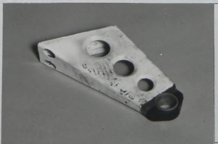
PHOTO No. 45 STABILIZER BAR BRACKET
