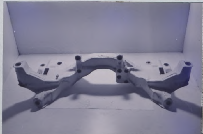
PHOTO No. 68 FRONT SUBFRAME
