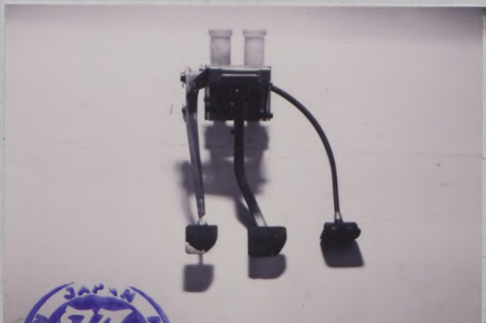
PHOTO No. 101 TWIN BRAKE MASTER CYLINDER
