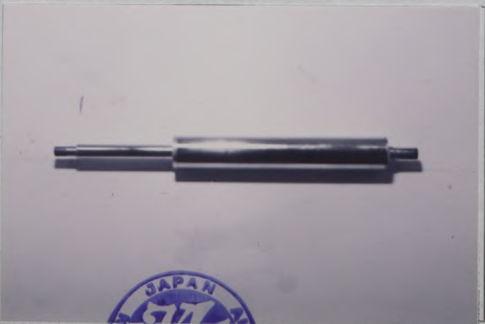
PHOTO No. 29 FRONT DAMPER UNIT
