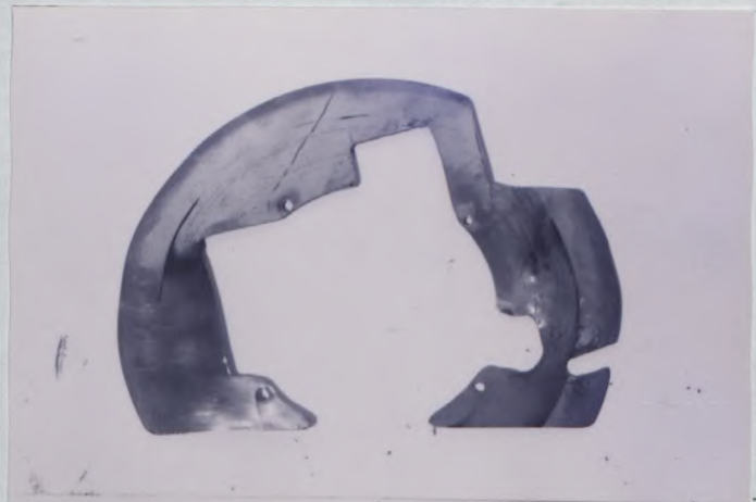
PHOTO No. 86 PROTECTION SHIELD FOR DISC
