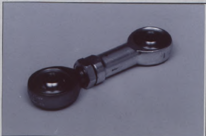
PHOTO N°3 STABILIZER BAR LINK
