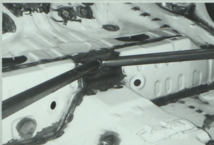
PHOTO N° 8 CENTRAL FRAMEWORK TO FLOOR
