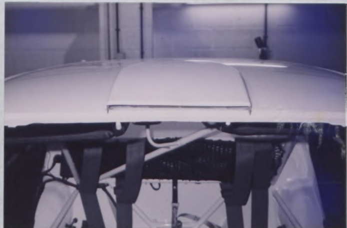
PHOTO No. 116 FLAPS FOR VENTILATION
