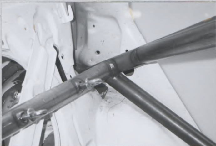
PHOTO No. 7 Rear longitudinal / Diagonal to bulkhead
