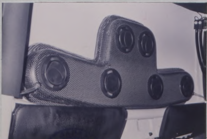
PHOTO No. 119 AIR VENT FOR FLAPS
