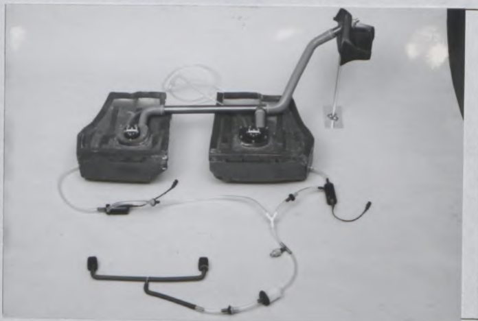
PHOTO No.121 DUAL WATER TANK
