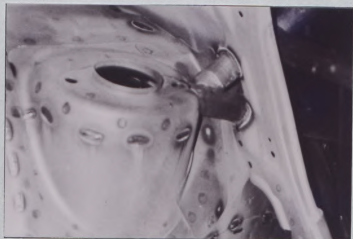
PHOTO No. 2 Rear longitudinal to rear turret
