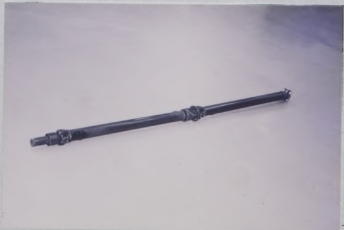
PHOTO No. 10 PROPELLOR SHAFT IN STEEL/STEEL
