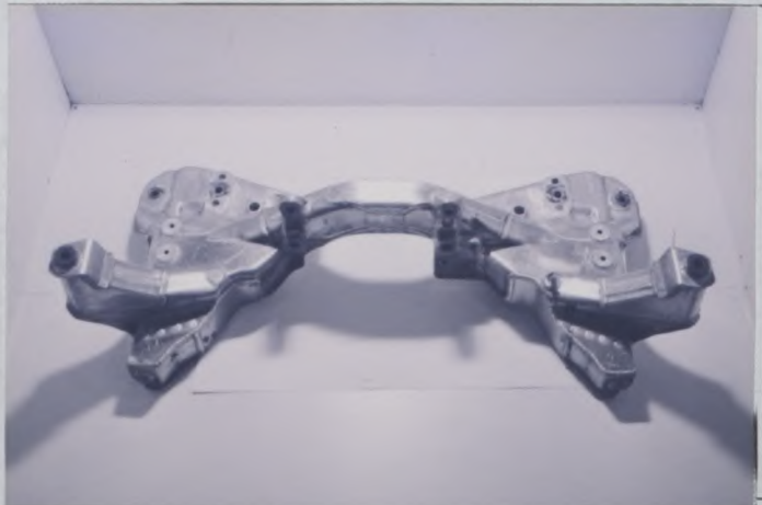
PHOTO No. 67 FRONT SUBFRAME
