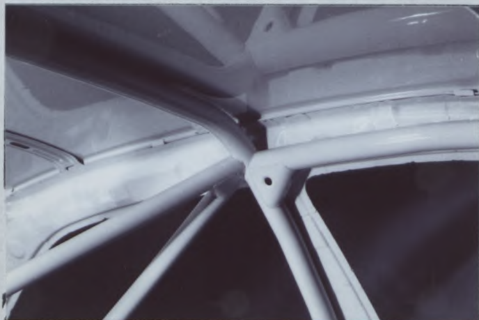
PHOTO N° 12 MAIN/LATERAL/DIAGONAL BAR JOINT
