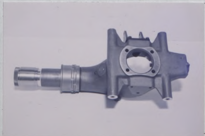
PHOTO No. 28 ALTERNATIVE UPRIGHT - FRONT
