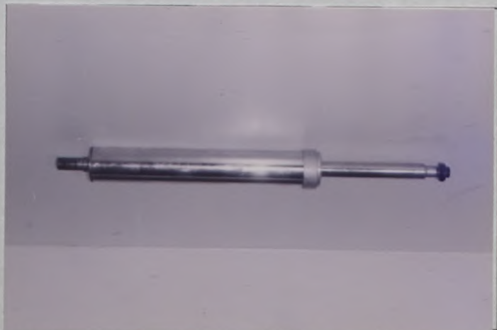
PHOTO No. 30 FRONT DAMPER UNIT
