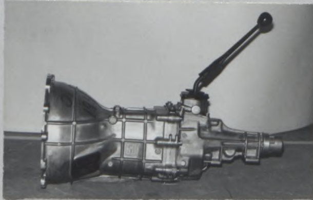
Photo H Gear-box profile
