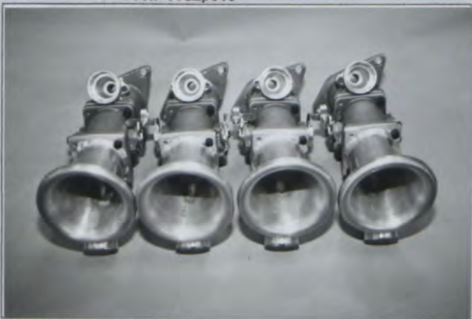
Photo No 1/8) Inlet manifold assembly complete with trumpets
