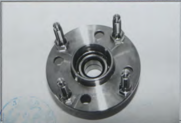
Photo No 17/98 Uprated wide track rear hub ----- Type D
