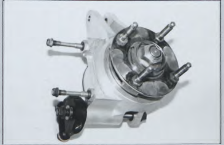
Photo No 16/98 Uprated front hub ----- Type C
