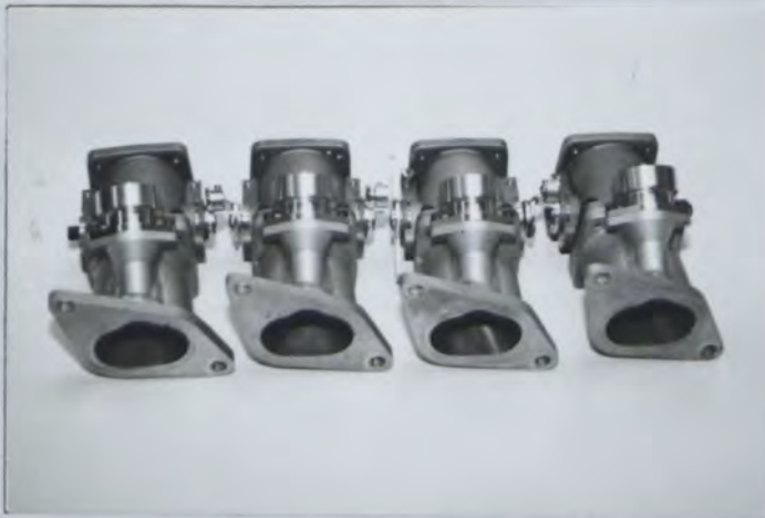
Photo No 1/8) Inlet manifold assembly complete with trumpets
