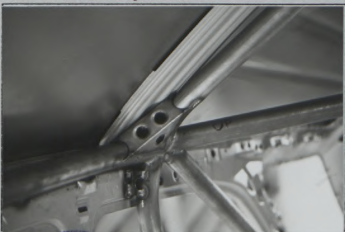
PHOTO No 5 Main hoop to roof
