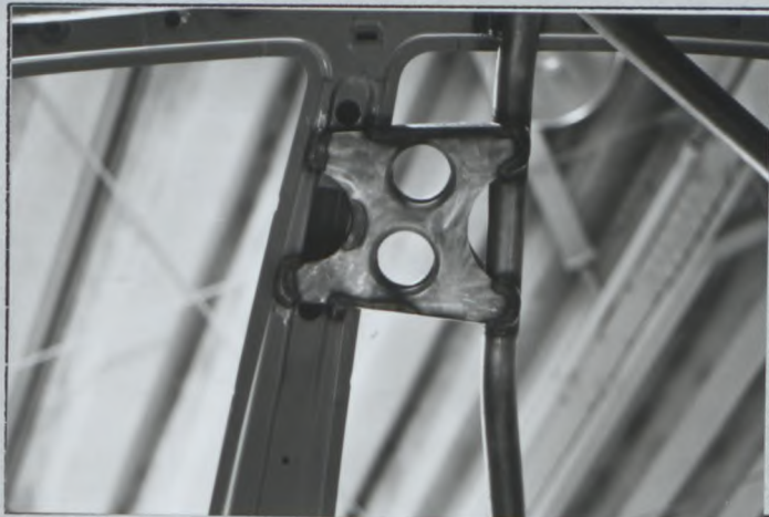
PHOTO No 7 Main hoop to pillar
