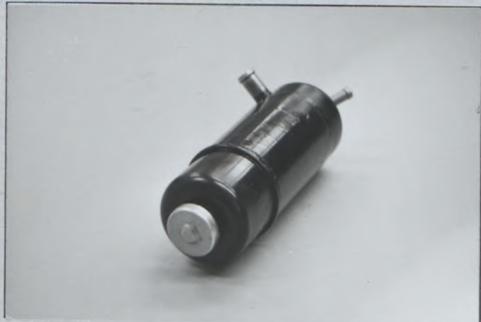
PHOTO No 1 STEERING FLUID RESERVOIR
