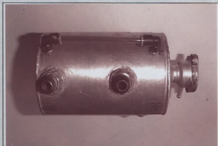
PHOTO No 4 STEERING FLUID RESERVOIR
