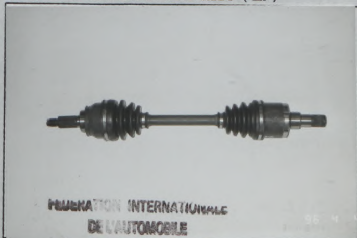
PHOTO No 6 REINFORCED DRIVE SHAFT ( LH )
