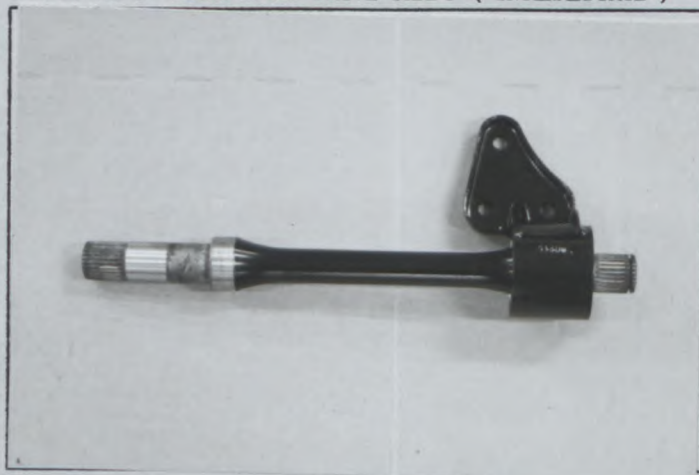
PHOTO No 8 REINFORCED DRIVE SHAFT ( INTERMEDIATE )
