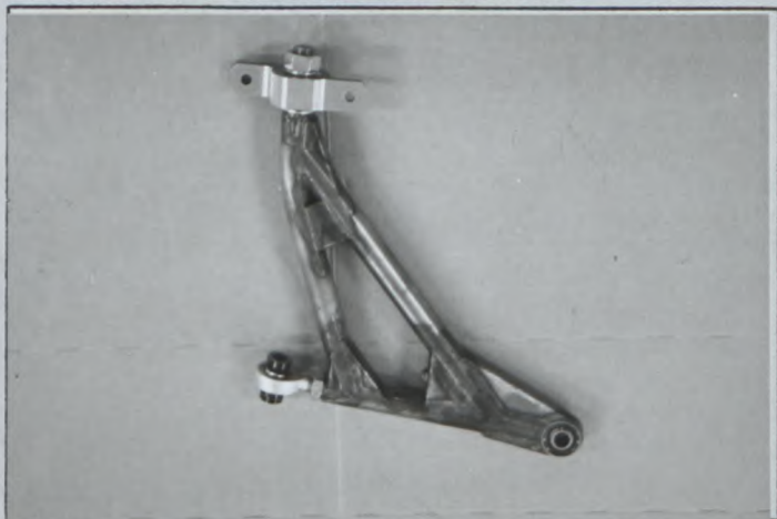
PHOTO No 13 REINFORCED FRONT LOWER ARM
