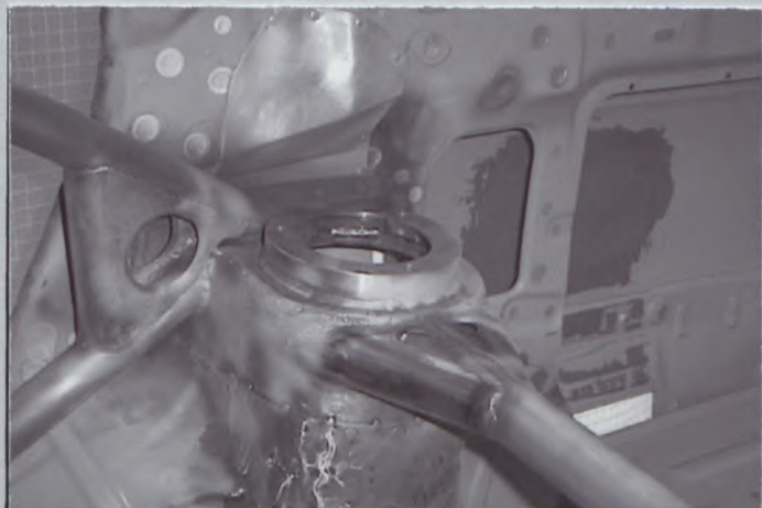
PHOTO N° 8 Rear support to turret
