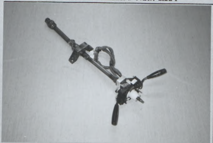
PHOTO No 37 REINFORCED STEERING COLUM SHAFT
