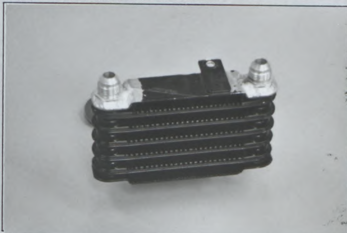
PHOTO No 2 STEERING FLUID COOLER
