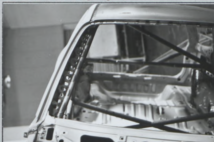
PHOTO No 2 Front hoop to pillar
