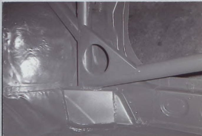
PHOTO N° 3 Front hoop to floor
