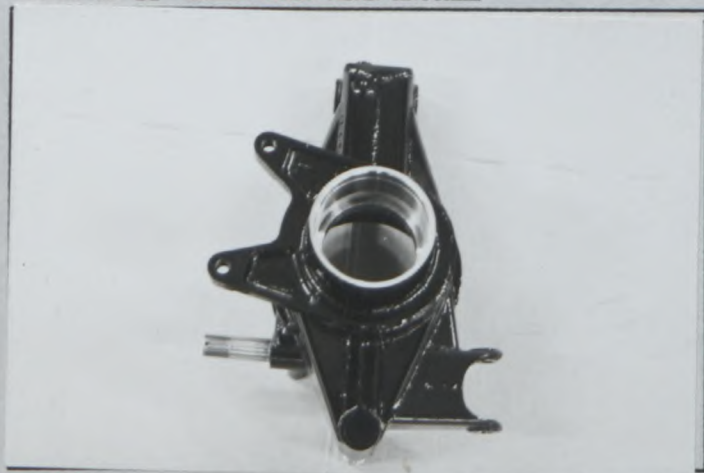
PHOTO No 21 REINFORCED REAR KNUCKLE
