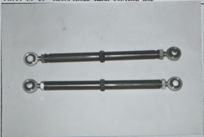
PHOTO No 15 REINFORCED REAR CONTROL ROD
