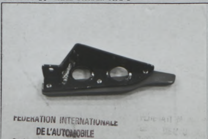
PHOTO No 24 WHEEL SCRAPER TYPE B
