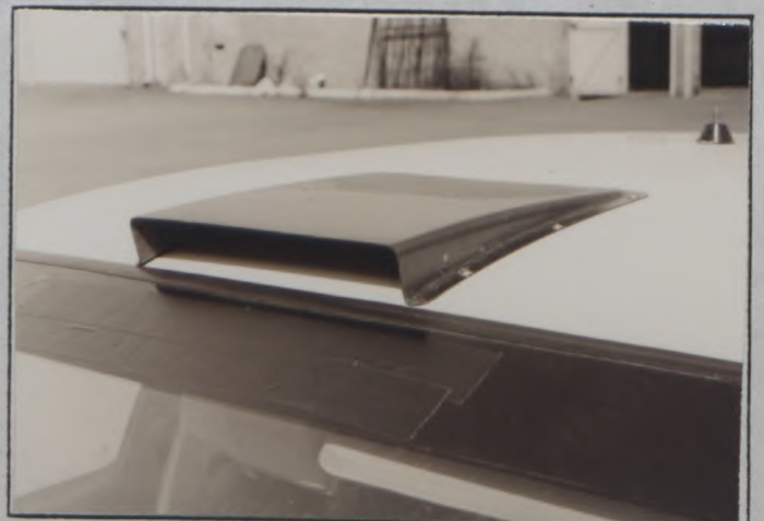
PHOTO No 96/26 Roof Ventilator (Ext)
