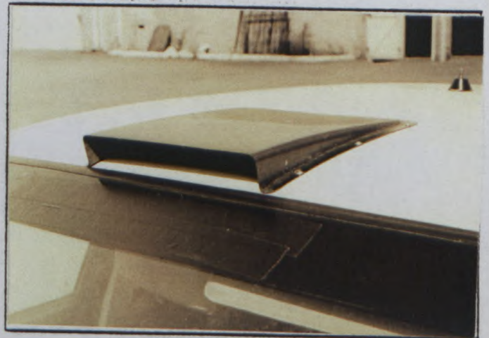
PHOTO No 96/26 Roof Ventilator (Ext)
