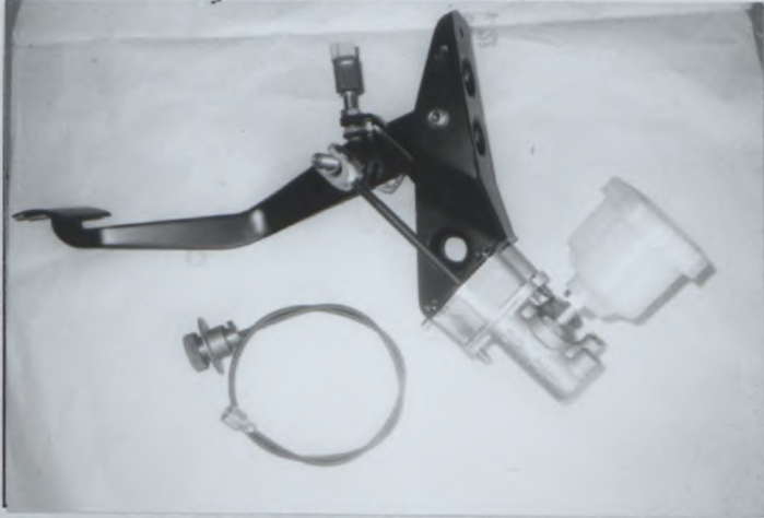
Photo No 45 Hydraulic hand brake control, TYPE A
