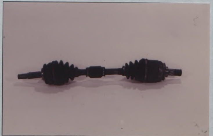
Photo No 6 Front reinforced drive shaft left hand, TYPE C
