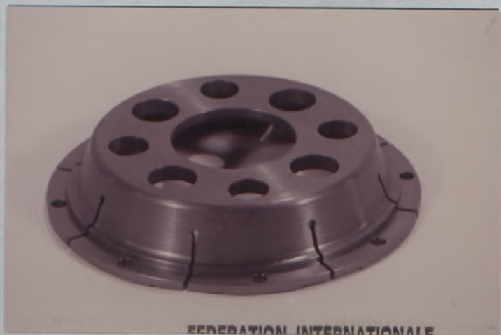
Photo No 54 Brake mounting bell, TYPE A
