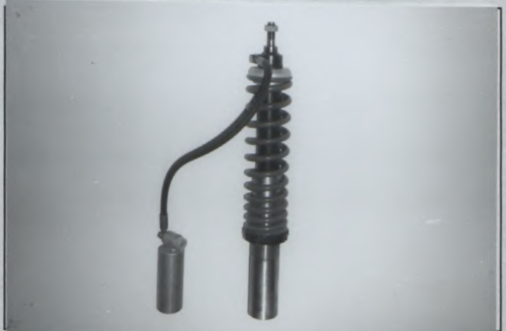
Photo No 36 Heavy duty rear shock absorber, TYPE A
