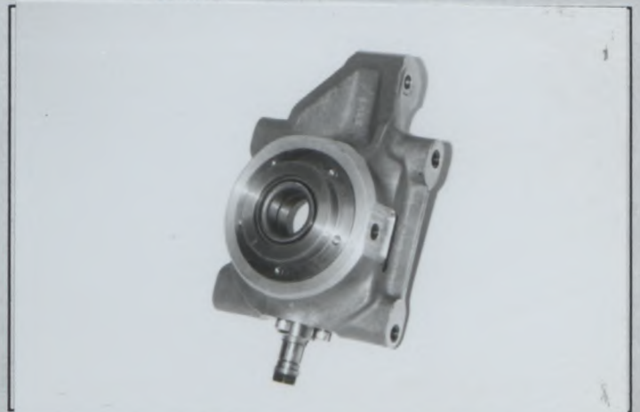
Photo No 12 Reinforced front upright left hand, TYPE C
