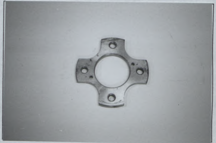
PHOTO No 40 Rear caliper mounting bracket, TYPE A
