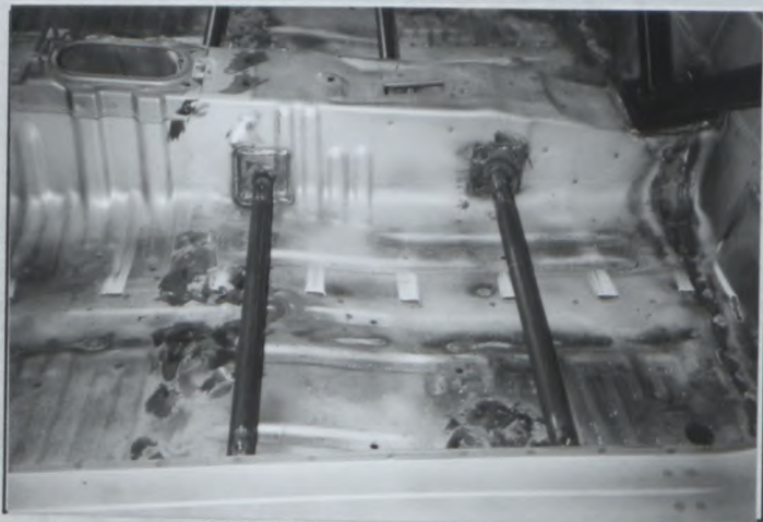
Photo No 75 Seat brackets, TYPE A
