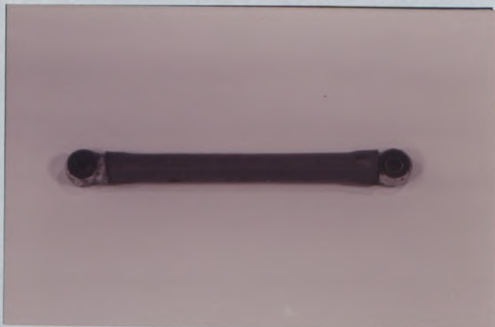
Photo No 28 Reinforced rear link lower, TYPE A
