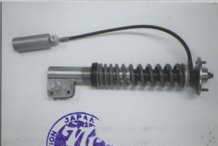
Photo No 35 Heavy duty front shock absorber, TYPE B
