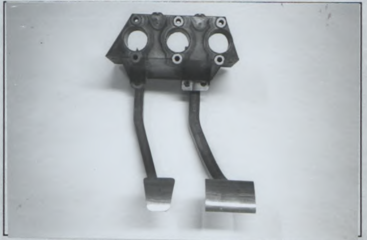
Photo No 46 Hydraulic hand brake control, TYPE B
