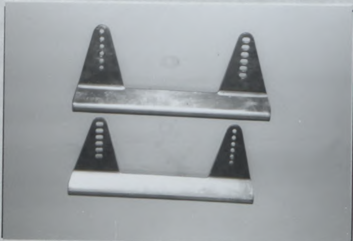
Photo No 75 Seat brackets, TYPE A
