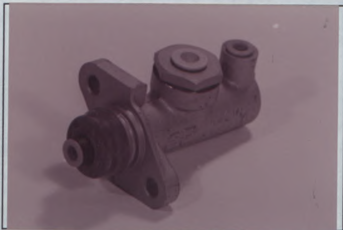
Photo No 51 Proportioning valve, TYPE A
