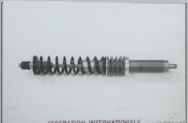
Photo No 36 Heavy duty rear shock absorber, TYPE A
