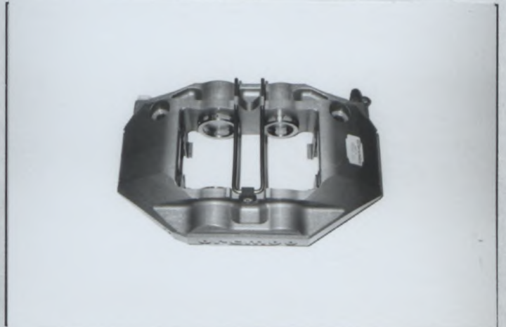
Photo No 58 Front caliper, TYPE C
