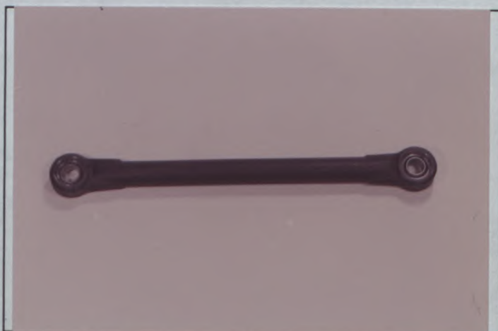
Photo No 30 Reinforced panhard rod rear, TYPE A
