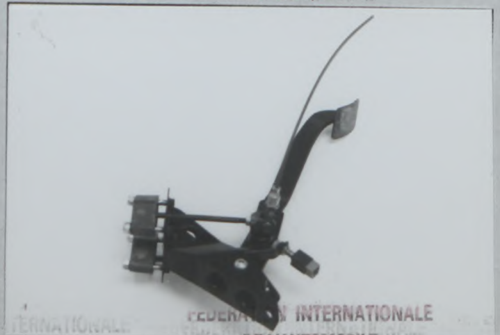
Photo No 42 Alternative brake pedal box with adjustable brake bias, TYPE A
