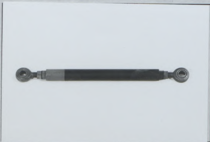
Photo No 29 Reinforced rear link lower, TYPE B
