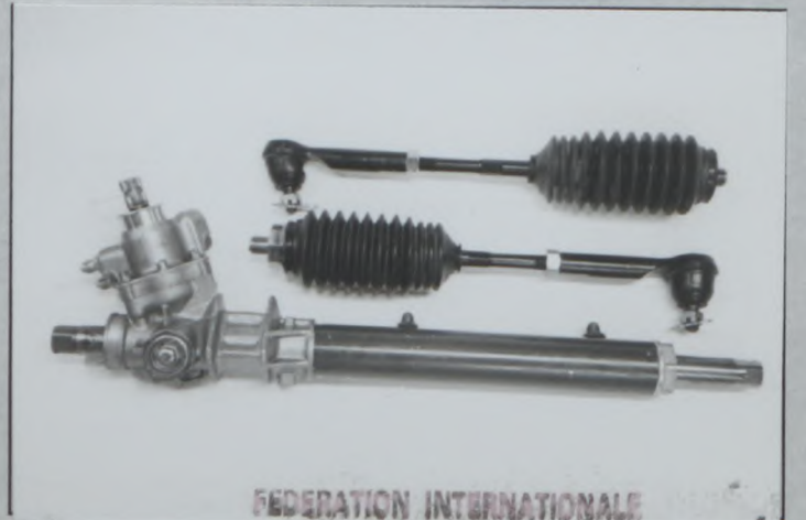
Photo No 66 Heavy duty steering gear and side rods, TYPE A
