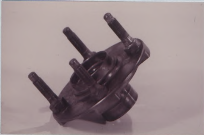
Photo No 15 Reinforced rear wheel hub, TYPE A
