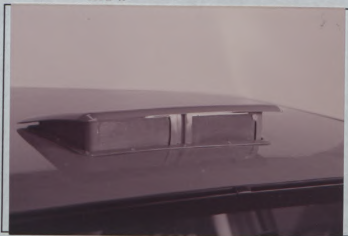
Photo No 76 Additional roof vent(for rallies only), TYPE A
