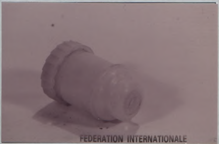
Photo No 48 Master/sub master cylinder reservoir tank, TYPE B
