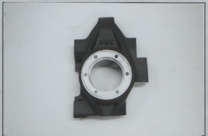
Photo No 12 Reinforced front upright left hand, TYPE C
