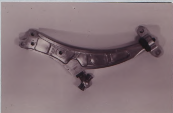
Photo No 24 Reinforced rear stabilizer with linkage, TYPE A
