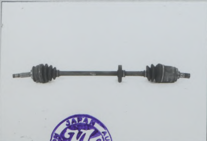
Photo No 5 Front reinforced drive shaft right hand, TYPE C
