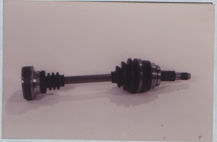
Photo No 4 Front reinforced drive shaft left hand, TYPE B
