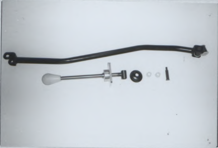
Photo No 3 Front reinforced drive shaft right hand, TYPE B
