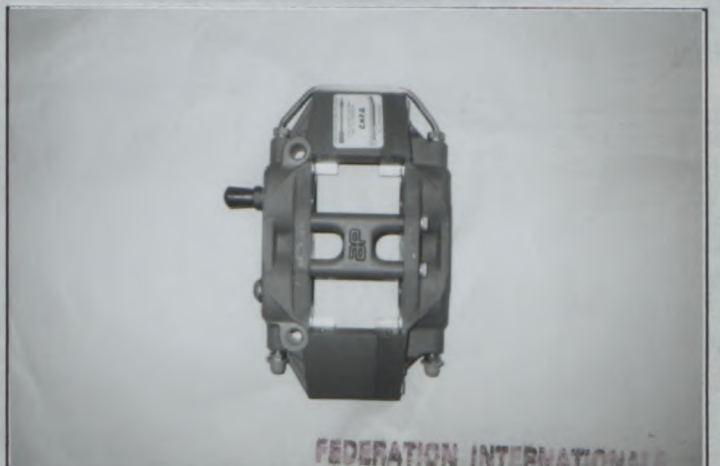
Photo No 60 Front caliper, TYPE E
