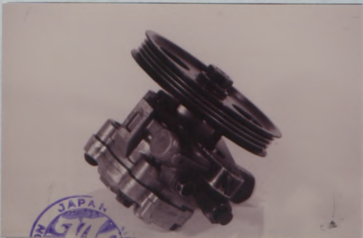
Photo No 71 Heavy duty power steering pump, TYPE A
