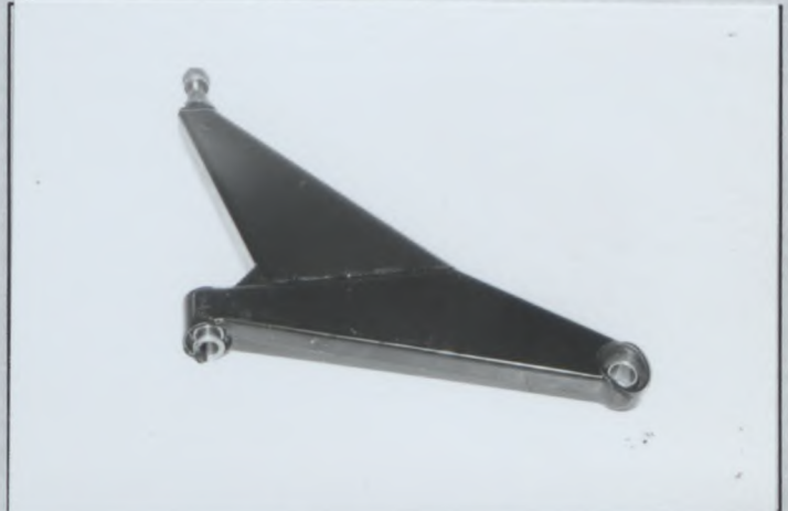
Photo No 22 Reinforced transverse link, TYPE C
