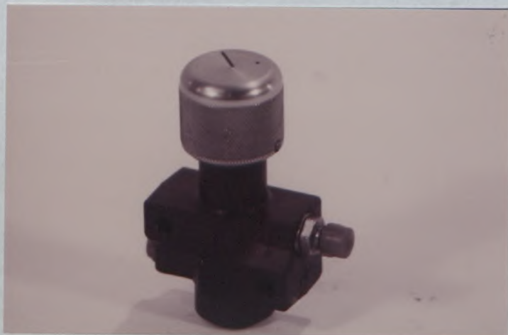
Photo No 53 Rear brake scraper, TYPE A
