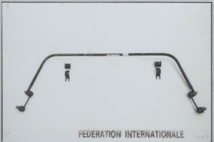
Photo No 24 Reinforced rear stabilizer with linkage, TYPE A
