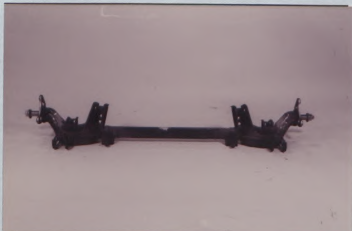
Photo No 27 Reinforced rear link upper, TYPE B
