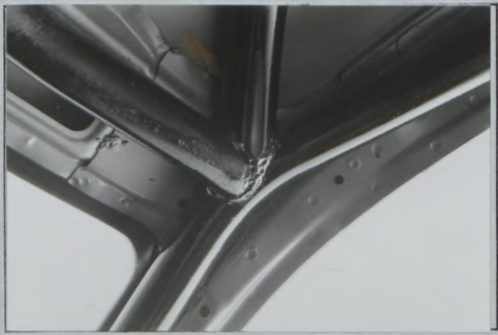
PHOTO No 5 Lateral Bar to A Pillar/ W/screen/roof Diagonal
