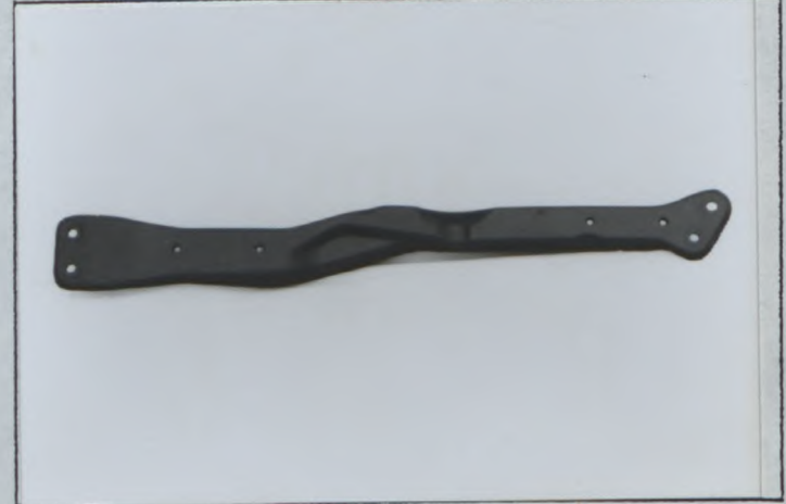
PHOTO No 28 Reinforced Front Longitudinal Member
