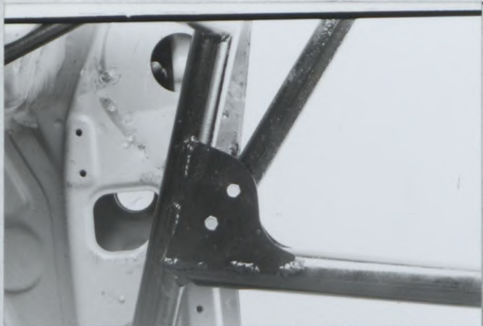
PHOTO No 7 Latéral Bar/brace/ side Intrusion to A Pillar
