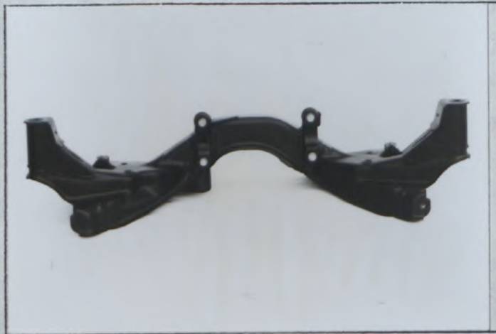
PHOTO No 27 Reinforced Front Subframe
