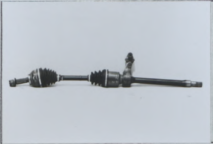
PHOTO No 3 Reinforced driveshaft, front (LH)
