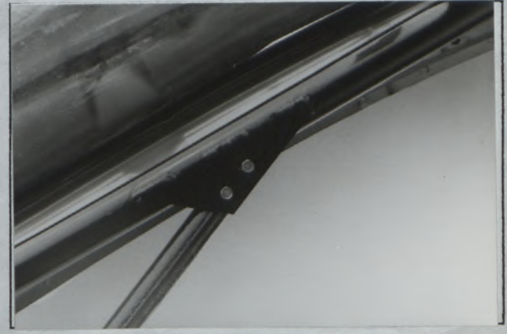
PHOTO No 6 Lateral Bar/Brace to A Pillar
