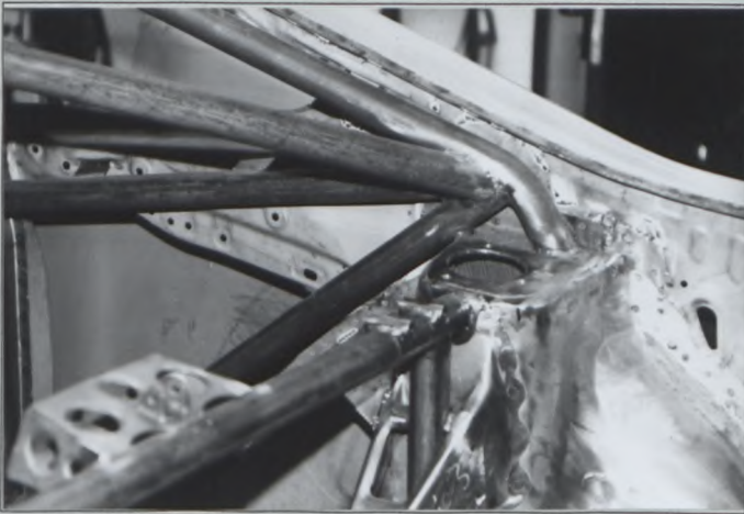
PHOTO No. 13 (REAR SUPPORT TO TURRET)
