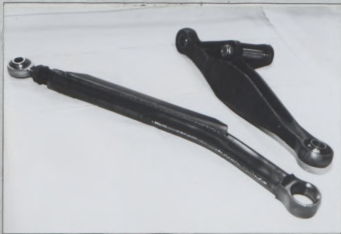
PHOTO NO. 9 (FRONT REINFORCED LOWER ARM)
