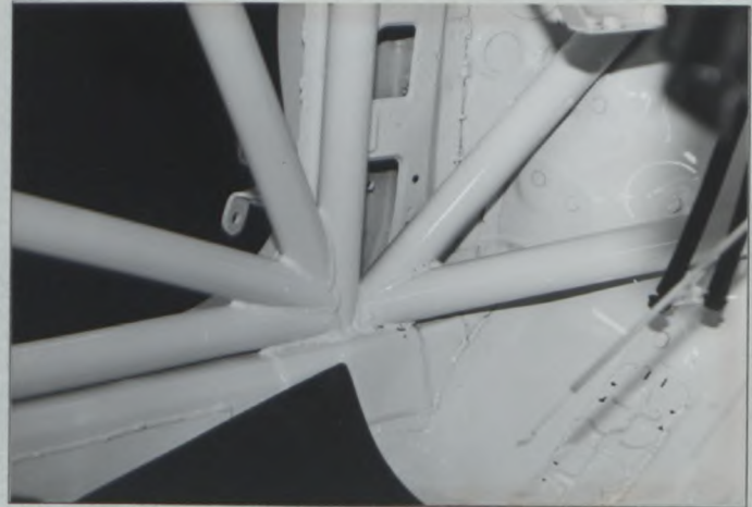
PHOTO No. 2 (FRONT HOOP TO FLOOR)
