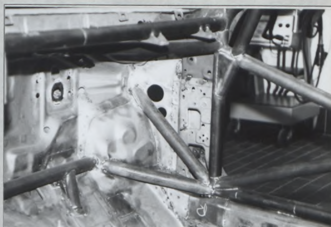
PHOTO No. 2 (FRONT HOOP TO FLOOR)
