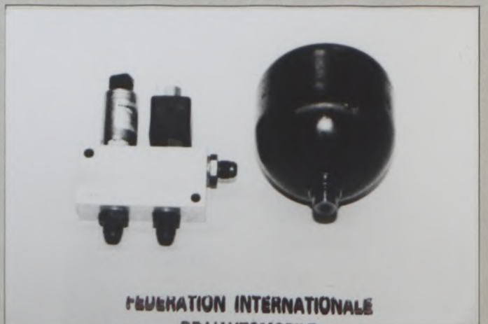
PHOTO NO. 6 (HYDRAULIC BOOSTER CONTROL UNIT : TYPE 2)
