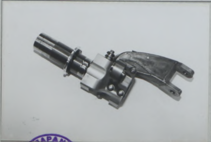
PHOTO 29 FRONT REINFORCED UPRIGHT (TYPE B)
