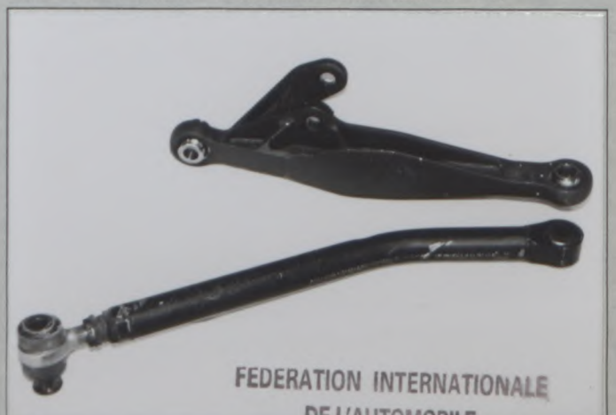
PHOTO NO. 6 (FRONT REINFORCED LOWER ARM:TYPE 2)
