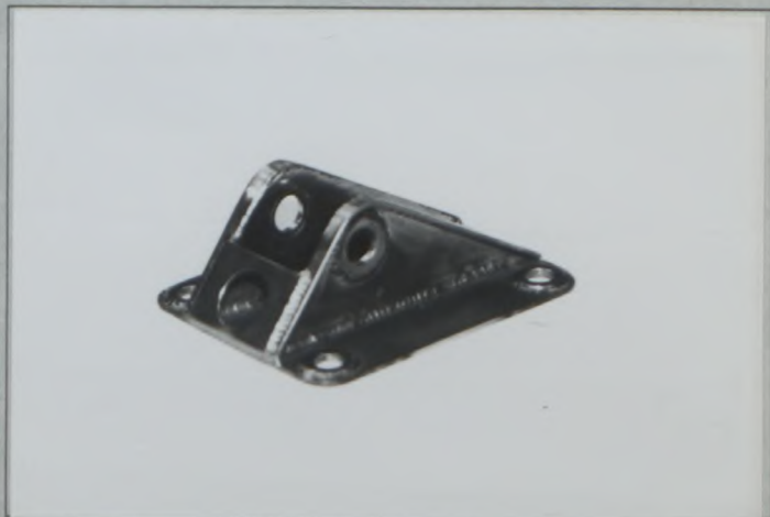
PHOTO 42 REINFORCED RADIUS ROD POINT (TYPE B)
