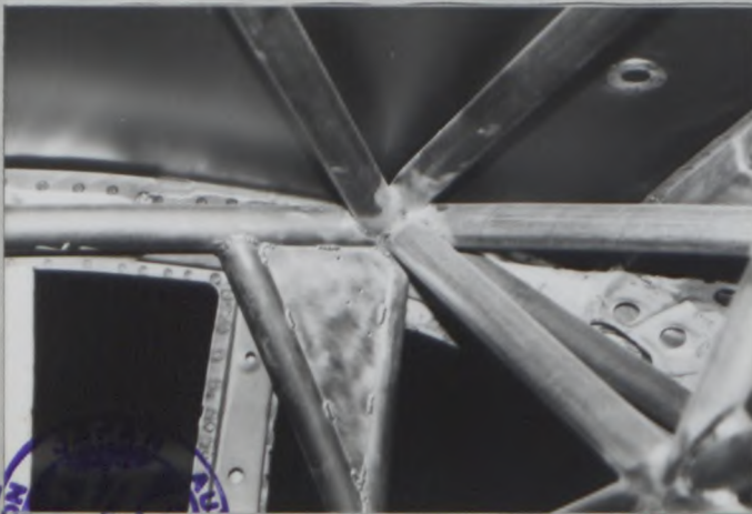
PHOTO No. 11 (MAIN HOOP TO ROOF)
