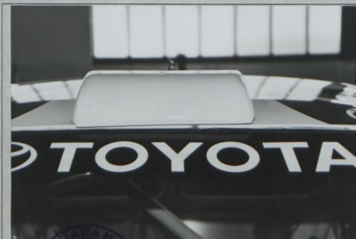
FLAPS FOR VENTILATION PHOTO 95
