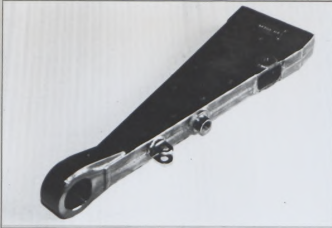
PHOTO NO. 1 (FRONT REINFORCED LOWER ARM)
