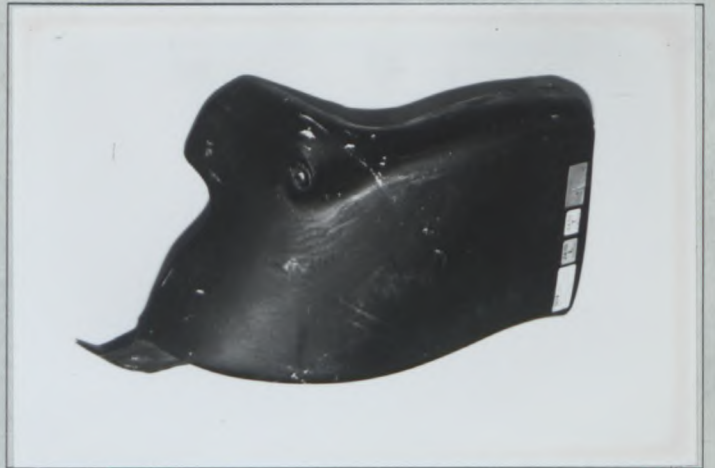
PHOTO 44 BRAKE COOLING DUCT
