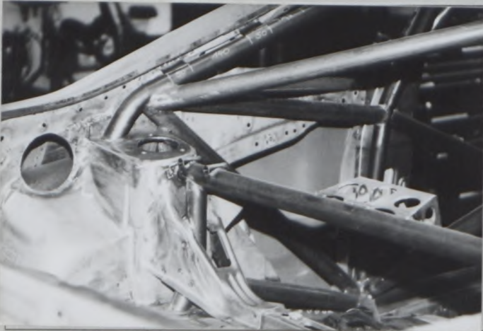
PHOTO No. 9 (REAR SUPPORT TO TURRET)
