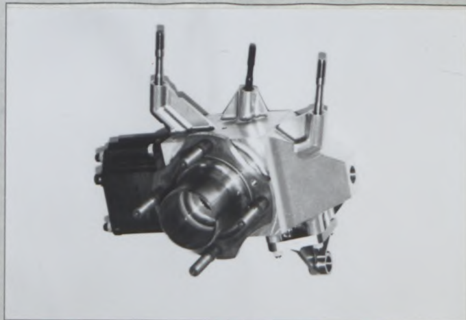
PHOTO NO. 10 (FRONT REINFORCED KNUCKLE)
