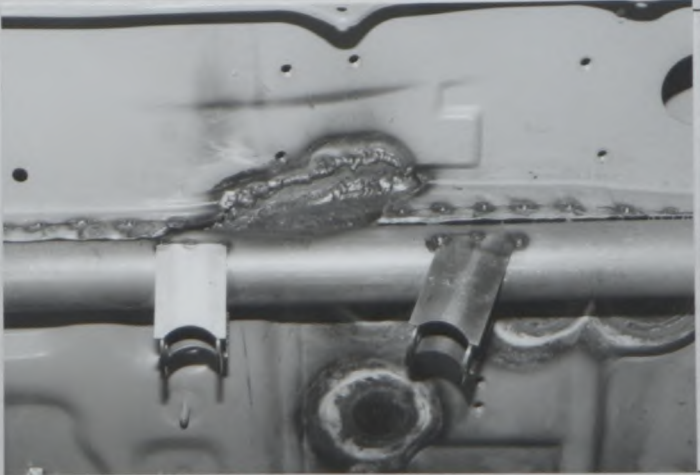
PHOTO No 17 Rear diagonal roll bars to shock absorber tower
