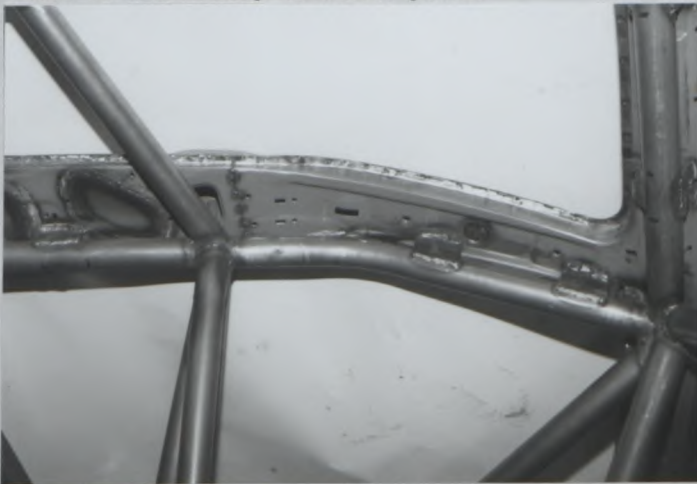
PHOTO No 11 Main diagonal roll bars to floor
