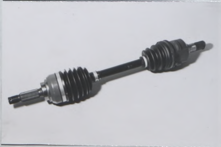
PHOTO No 3 REINFORCED DRIVESHAFT, FRONT (RH)
