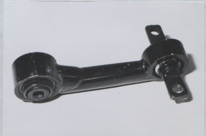
PHOTO No 16 REINFORCED TOE CONTROL LINK REAR
