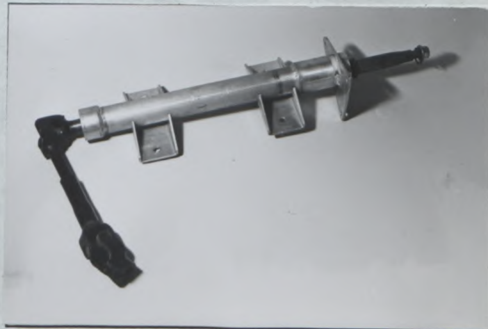
PHOTO No 52 REINFORCED STEERING COLUMN
