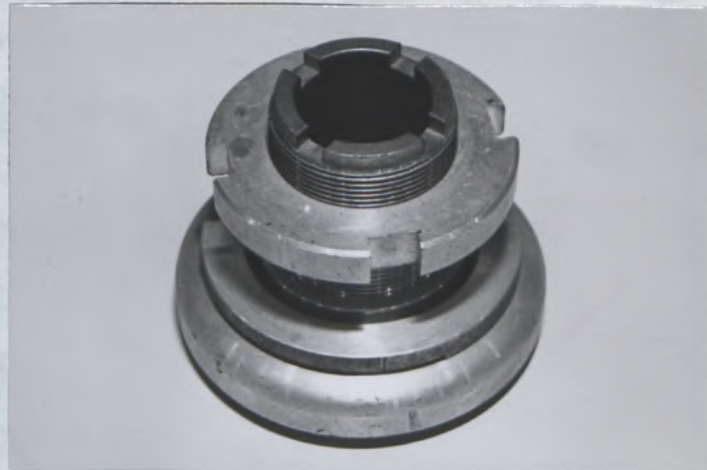
PHOTO No 20 REINFORCED STRUT TOP MOUNT TYPE 4
