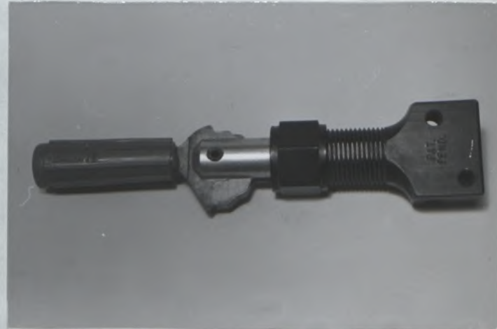
PHOTO No 34 PRESSURE CONTROL VALVE
