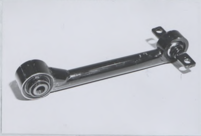
PHOTO No 13 REINFORCED UPPER TRANSVERSE LINK - REAR
