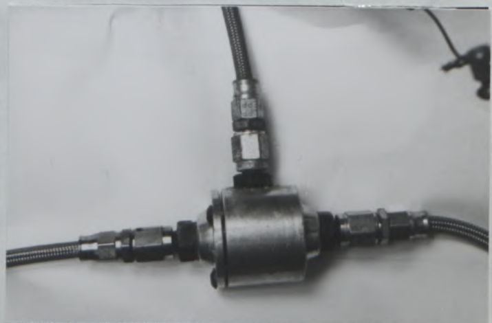
PHOTO No 30 FLUID DISTRIBUTION VALVE
