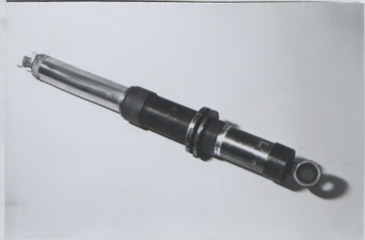
PHOTO No 26 LIQUID COOLED REAR SHOCK ABSORBER
