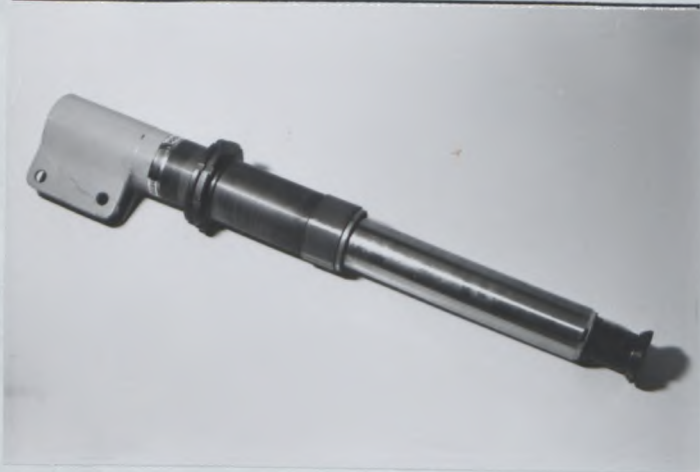
PHOTO No25 LIQUID COOLED FRONT SHOCK ABSORBER
