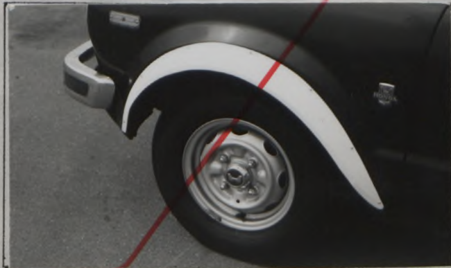
Photograph, Front wing extension
