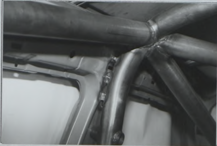
PHOTO No 11 Rear support bars to floor
