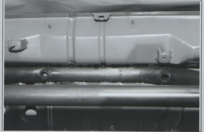
PHOTO No 4 Front hoop and Front lateral roll bar to dash upper, right hand
