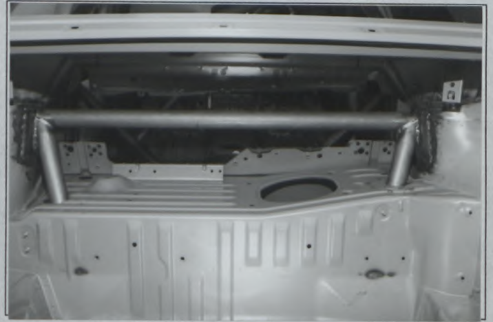
PHOTO No 16 Rear lateral bar and support bar to shock absorber tower, Rear side
