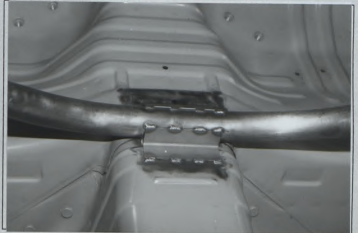
PHOTO No 12 Front support bar to shock absorber tower
