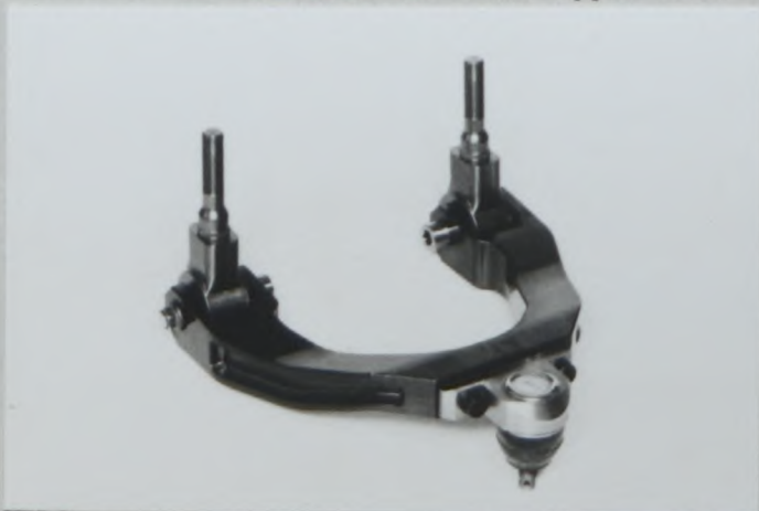
PHOTO No T3 Reinforced front upper arm
