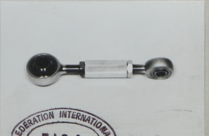
PHOTO No T12 Reinforced rear compensator arm
