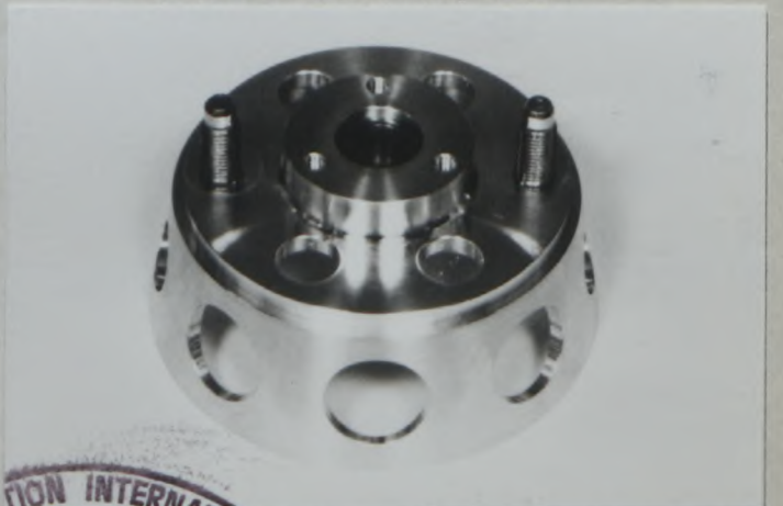
PHOTO No T6 Reinforced front damper mount
