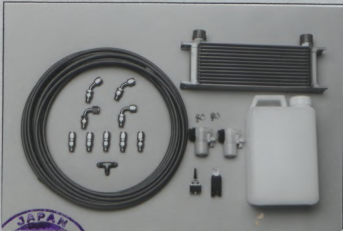
PHOTO No V1 Kit brake water cooling system
