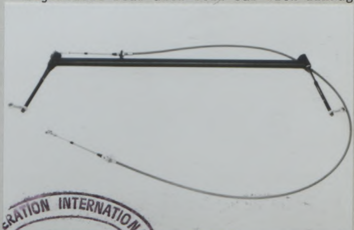
Adjustable rear anti-roll bar with linkage
