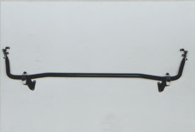
PHOTO No T9 Front anti-roll bar with linkage
