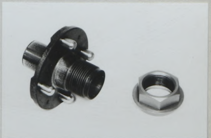
PHOTO No T10 Front hub for center lock
