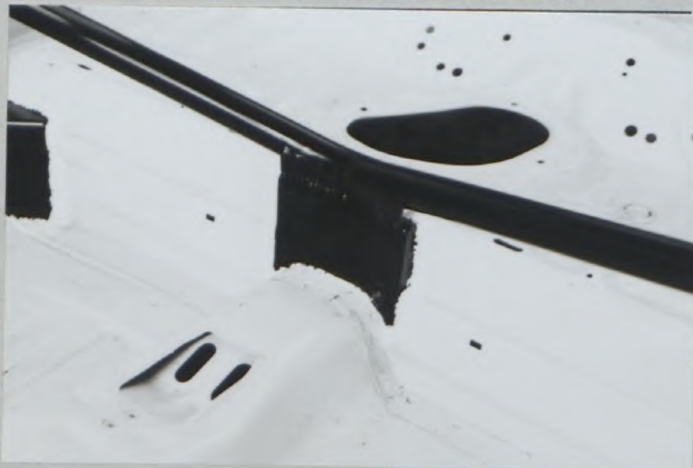
PHOTO Main lateral rollbar to floor
