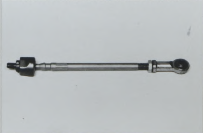
PHOTO No V7 Reinforced steering tie-rod type 1
