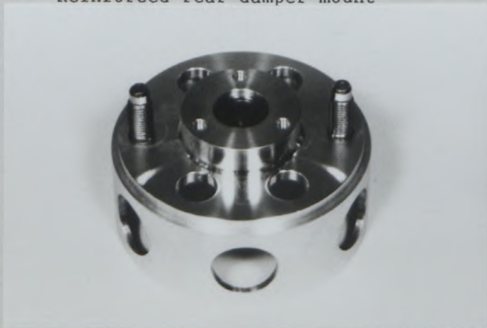
Reinforced rear damper mount
