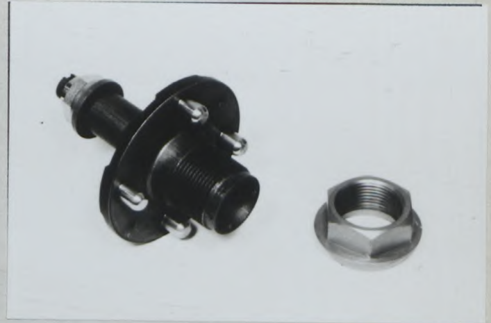
PHOTO No T20 Rear hub for center lock 1/1
