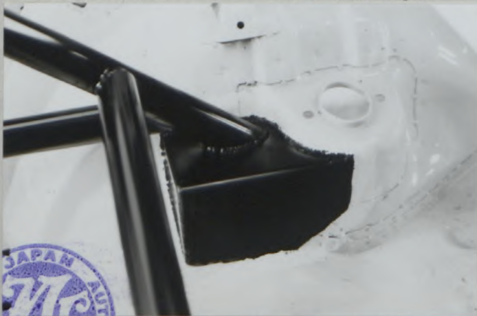
PHOTO Rear support bar to damper house right
