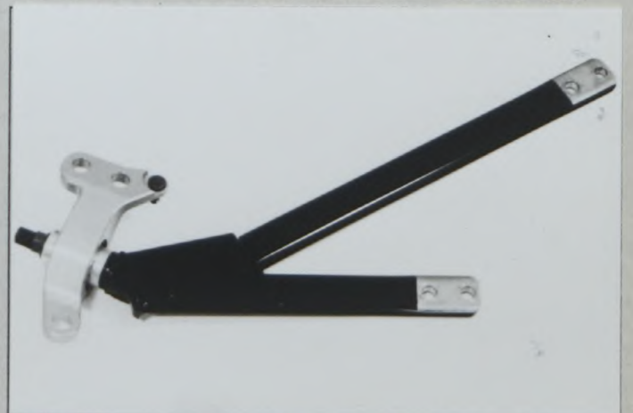
PHOTO No T4 Reinforced front radius arm
