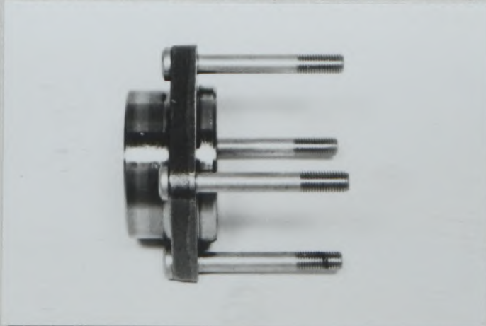
PHOTO No T21 Heavy duty rear hub bearing
