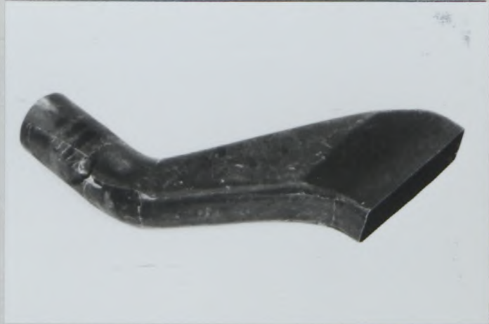
PHOTO No V5 Front brake cooling air intake type 1
